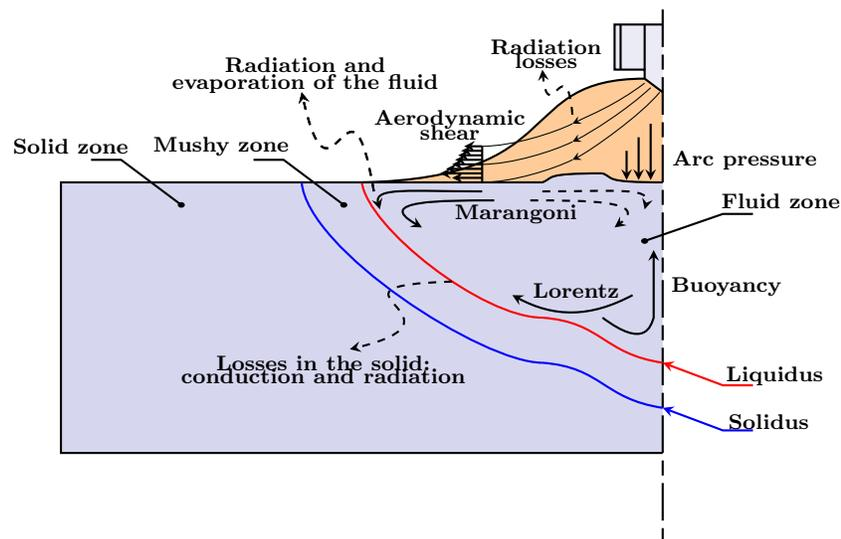
Figure 1: *Schematisation of the material states and the fluid flows during welding process*
