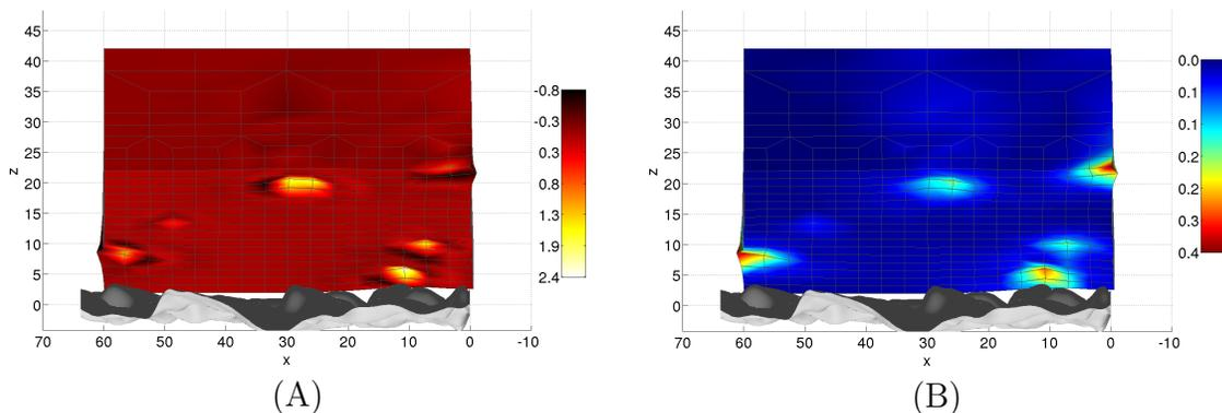
Figure 1: (A) Temperature distribution and (B) visco-elastic strains in the tread block after contact with rough surface.
