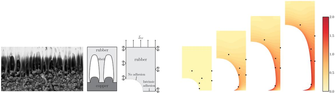
Figure 2: (Left) Fibrils connected to substrate in roughness valleys, the idealized representation and the single fibril model. (Right) Several stages of the fibrillation process. Colors indicate maximum principal true strain. The large displacement of material points is tracked by the dots.
