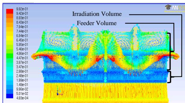
**Fig 2: Velocity-vectors plot [m/s] - uniform distribution at outlet apertures**
