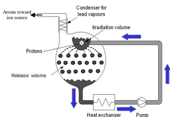
Fig 1: Conceptual view of circulating LBE target
