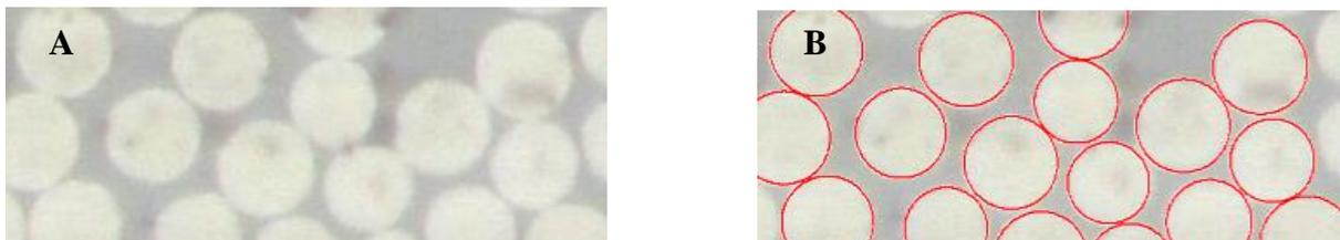
**Figure 1:** (A) Original image of microstructure from light microscope. (B) Sample of analysed image with fibres automatically located for input into finite element analysis software.
