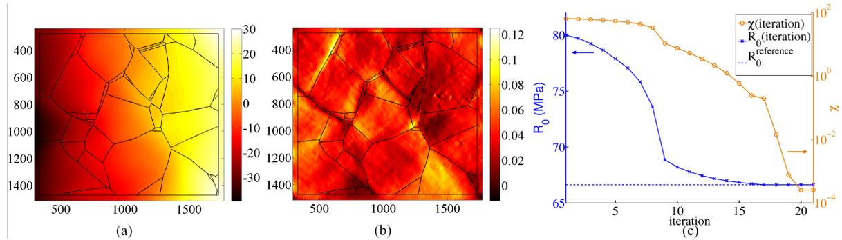
Figure 1: Longitudinal displacement field in pixels (a) and longitudinal strain field (b) measured experimentally for a macroscopic strain of 5%. The physical size of one pixel is 150 nm. The grain boundaries are shown as black lines on these fields. Change of the cost function  $\chi$  and of the critical resolved shear stress  $R_0$  as functions of the iteration of the identification procedure (c). In this test case, a set of reference values of parameters is to be identified.
