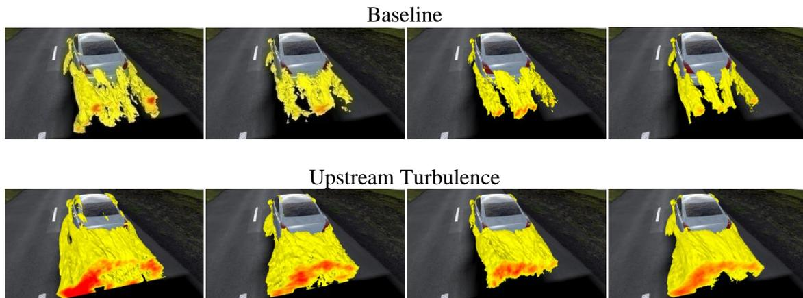
Figure 1. Velocity fluctuations in the region around the vehicle are shown using isosurfaces of turbulence intensity. From left-to-right the images show X-velocity fluctuations ( $I_x$ ), Y-velocity fluctuations ( $I_y$ ), Z-velocity fluctuations ( $I_z$ ), and total turbulence intensity ( $I$ ), each with value 15%. The lack of symmetry in the wake is due to low-frequency fluctuations coming from the upstream turbulence.
