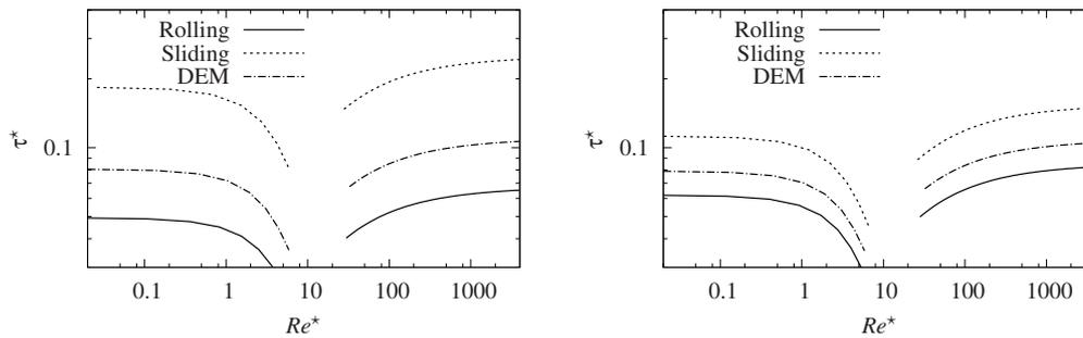
Figure 2:  $Re^*-\tau^*$  relation for an spherical (left) and ellipsoidal particles (right) with the analytical and numerical (DEM) approaches.
