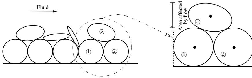
Figure 1: Sediment bed with composed by the repetition of the simple pattern of spheres on the bottom and a series of ellipsoids on the top with an stable orientation (right)
