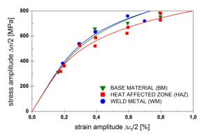
**Figure 3**: Cyclic stress-strain relation of the three zones BM, HAZ and WM for a S960QL butt weld (preliminary results)
