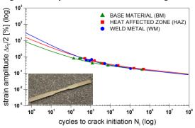
**Figure 2**: Strain-life of the three zones BM, HAZ and WM for a S960QL butt weld (preliminary results)
