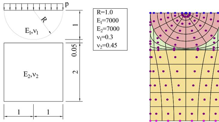
**Figure 1:** Geometry and coarse mesh for the Hertzian contact problem.
