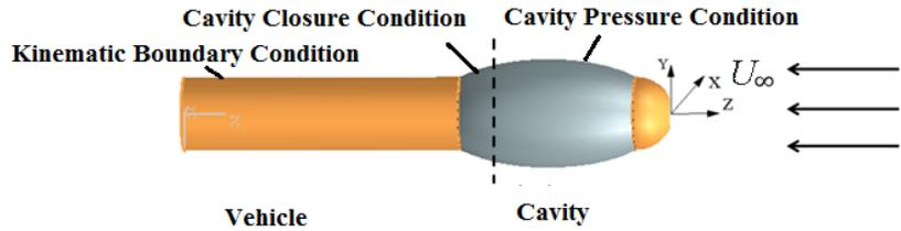
Figure 2: The model for the calculation of vehicle with partial cavity flow
