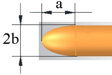
**Figure 5:** The Sketch of different head shapes' parameters
