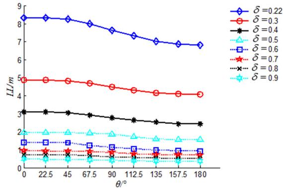
**Figure 6:** The circumferential curve of cavitation length under different cavitation number
