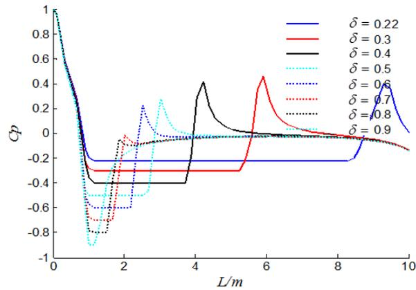
**Figure 10:** The curve of  $C_p$  at back flow surface under different cavitation number
