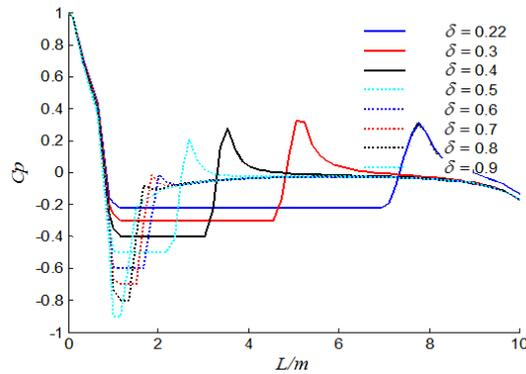
Figure 9: The curve of  $C_p$  at front flow surface under different cavitation number
