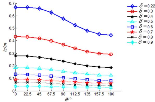
**Figure 7:**The circumferential curve of cavitation maximum thickness under different cavitation number
