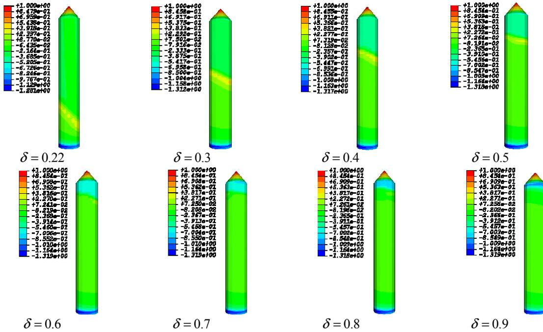
Figure 8: The nephogram of  $C_p$  under different cavitation number
