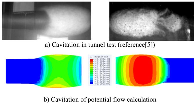
**Figure 3:** The contrast of cavitation between calculation and tunnel test (Left is front flow surface)
