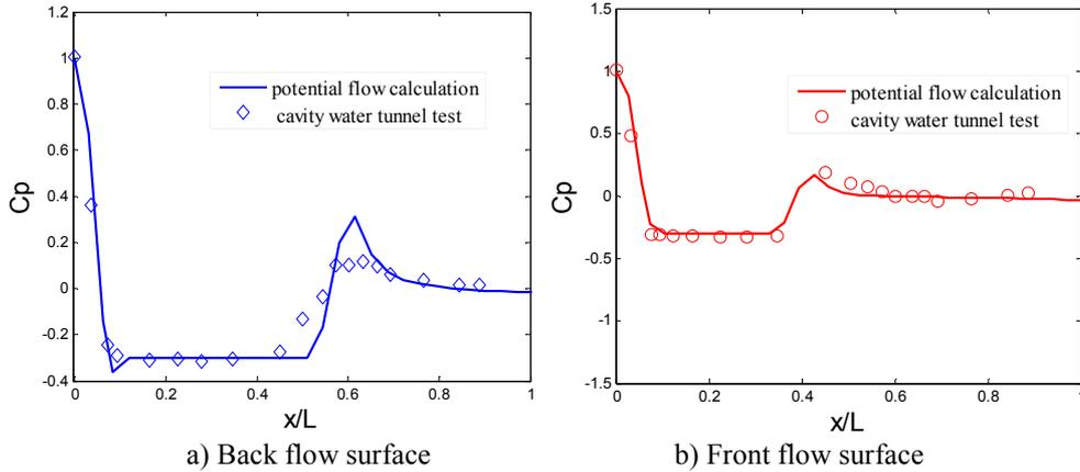
**Figure 4:** The compare of  $C_p$  between Potential flow calculation and tunnel test
