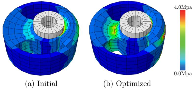
**Figure 3:** Comparison of von Mises stress
