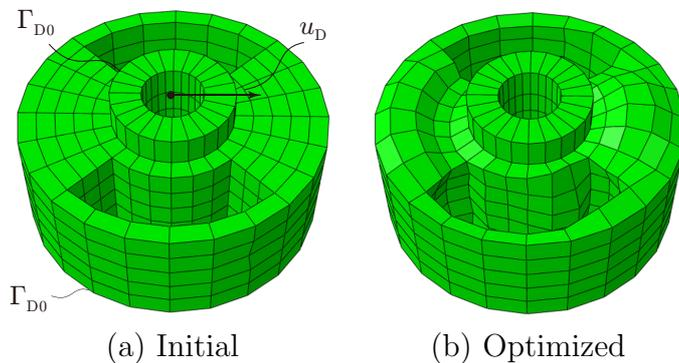
**Figure 1:** Finite element models of simple rubber bushing
