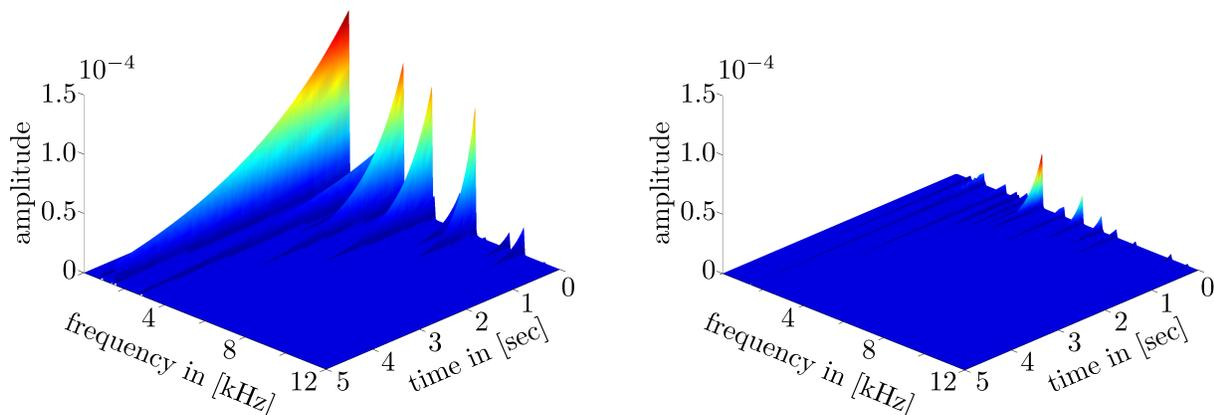
Figure 6: Spectrograms for the high-quality triangle (left) and the low-quality triangle instrument (right).
