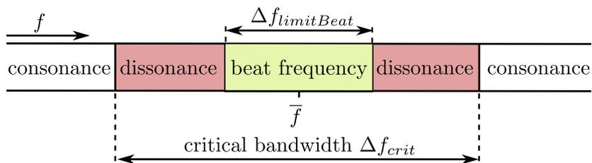
Figure 2: Partition of the critical bandwidth into the dissonant area and the area of beat frequency.
