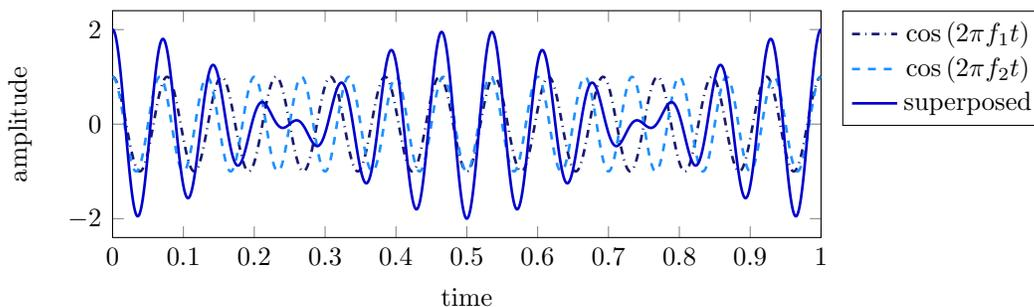
Figure 3: Beat frequency occurring by the superposition of two tones with a frequency difference of 2 Hz.
