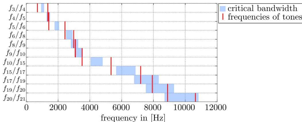
Figure 9: Critical bandwidth between two neighboring frequencies of the spectrum of the low-quality triangle.
