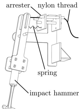
Figure 5: Mounting of the impact hammer.
