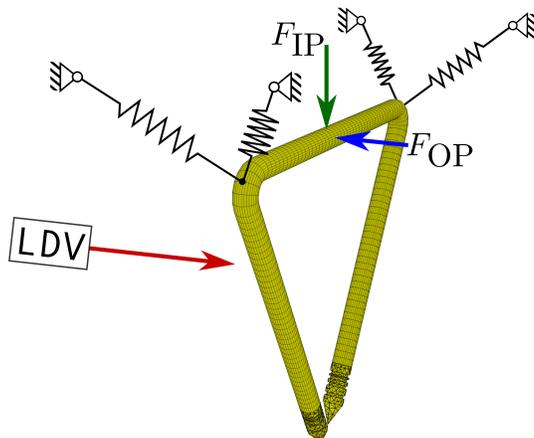
Figure 4: Suspension and excitation directions of the triangle instrument.
