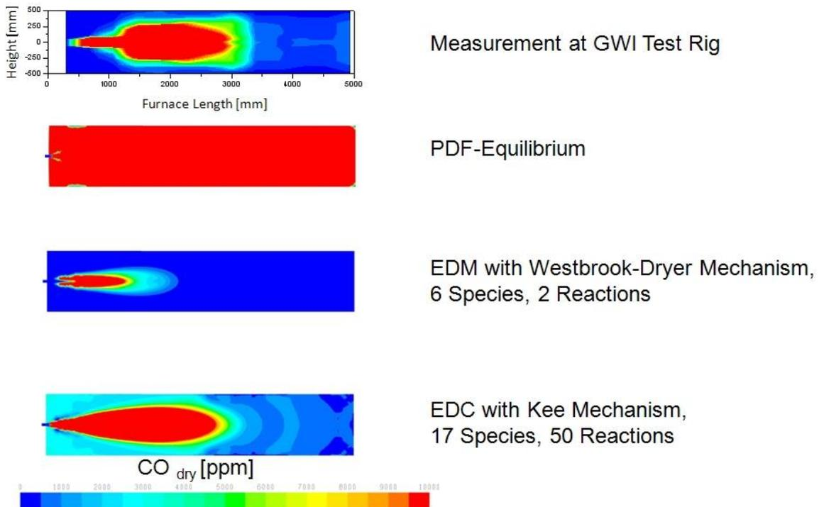
Figure 7: Comparison of measured and simulated CO concentration distributions
