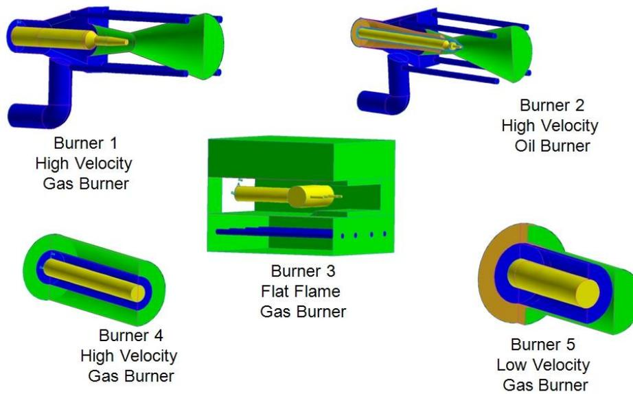
Figure 1: Sketches of the investigated oxy-fuel burners
