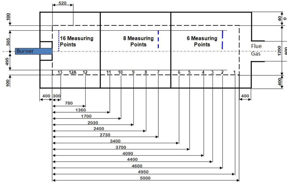
Figure 3: Measuring plan of GWI's semi-industrial test rig
