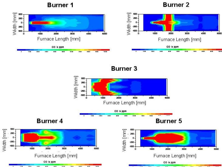
Figure 4: Measured CO distributions for the investigated burners
