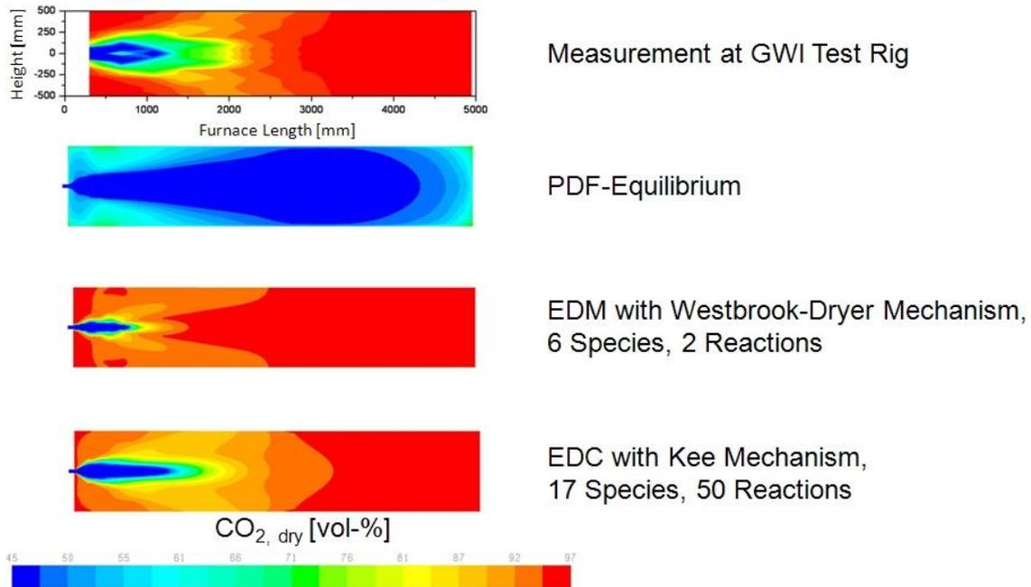
Figure 6: Comparison of measured and simulated CO<sub>2</sub> concentration distributions
