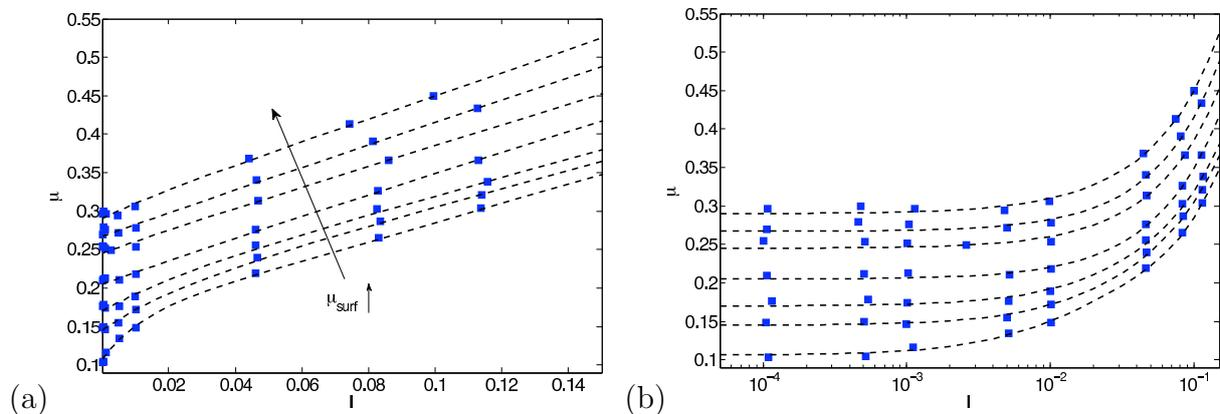
**Figure 3:** Planar shear flows: DEM data (squares) and selected fit functions per Equation 5 (dashed lines) corresponding to all seven particle surface frictions, displayed simultaneously in (a) linear and (b) semilog.
