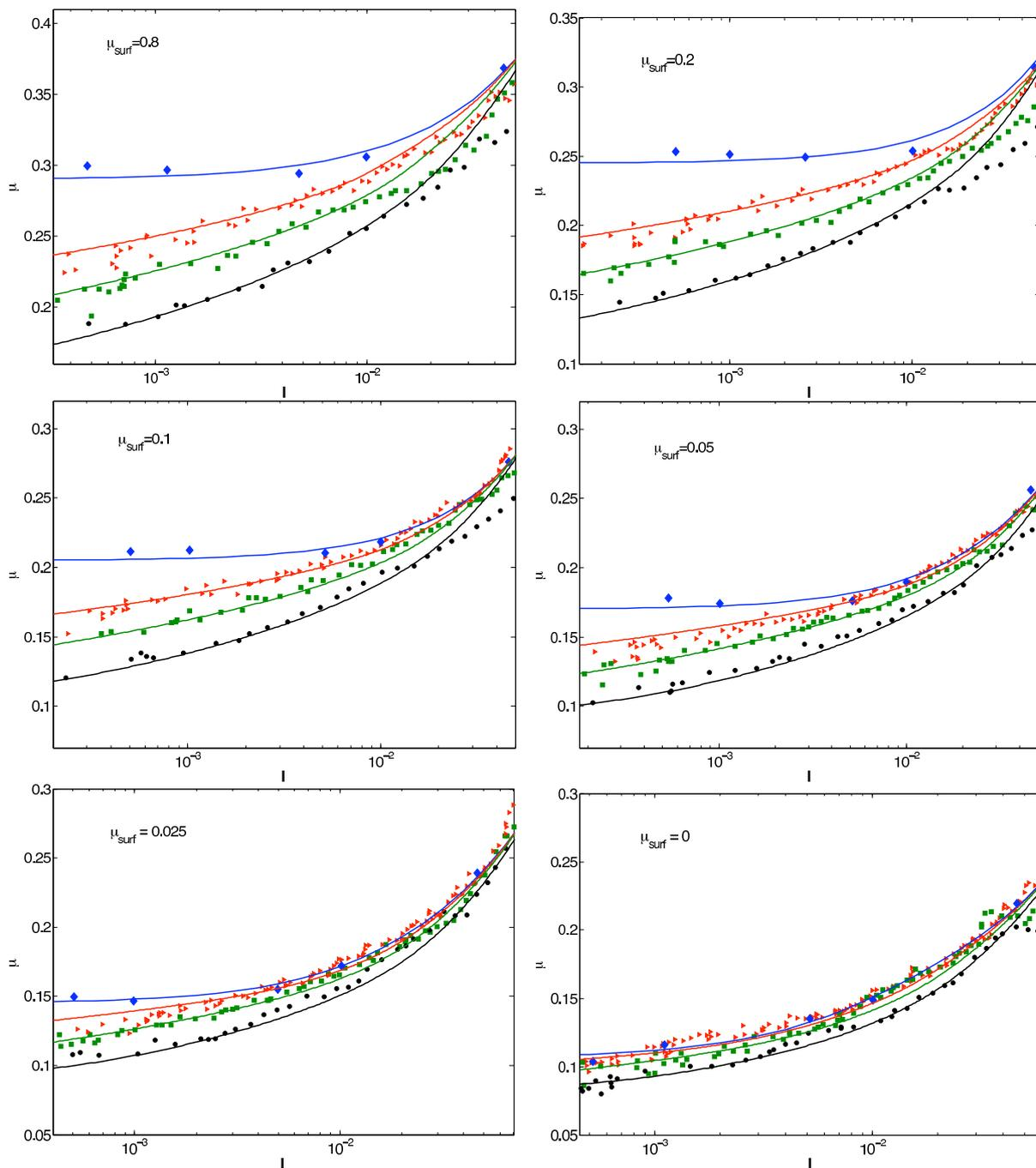
**Figure 4:** Calibrated NGF model [c.f. Table 2] (lines), vs DEM data (symbols) for planar shear ( $\blacklozenge$ ) and annular shear geometries with  $R = 25d$  ( $\bullet$ ),  $50d$  ( $\blacksquare$ ),  $100d$  ( $\blacktriangleright$ ).
