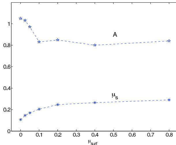
**Figure 5:** Dependence of the nonlocal amplitude and the static planar shear strength on surface friction.
