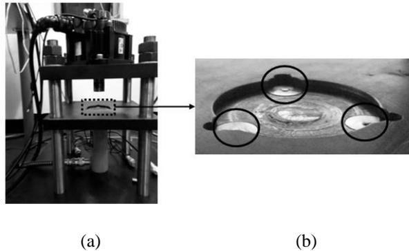
**Figure 2:** (a) Bearing wear test equipment (b) Locations of three load cells
