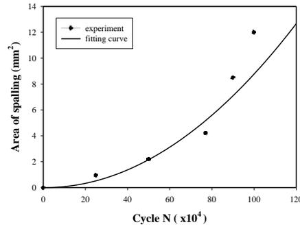
Figure 5: Experiment result of spalling test for bearing
