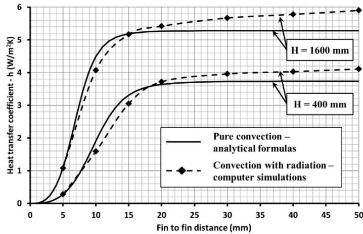
Figure 5: The influence of radiation on overall heat transfer coefficient.
