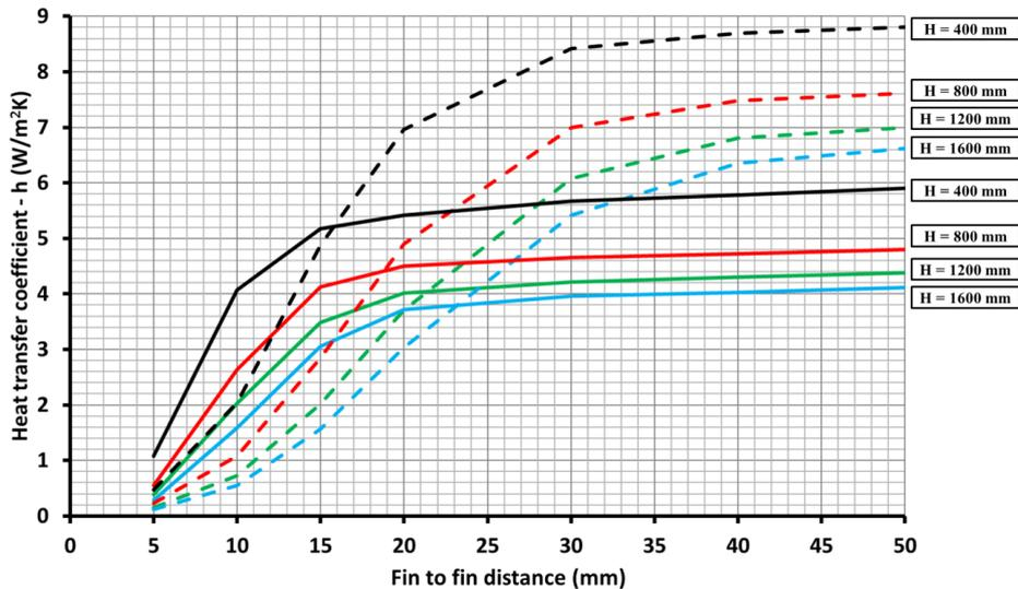
**Figure 7:** The comparison of the cooling efficiency of the heat sink without and with panels.
