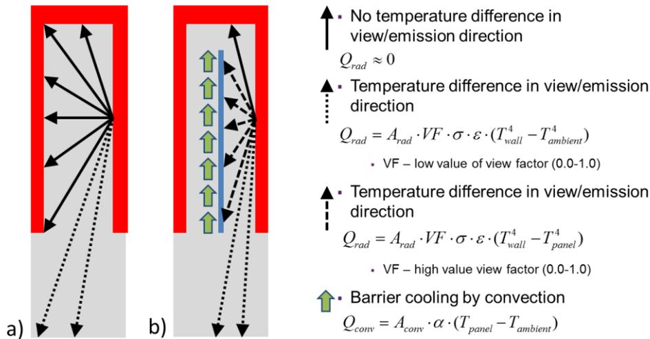
**Figure 4:** Heat transfer by radiation in heat sinks with fins.
