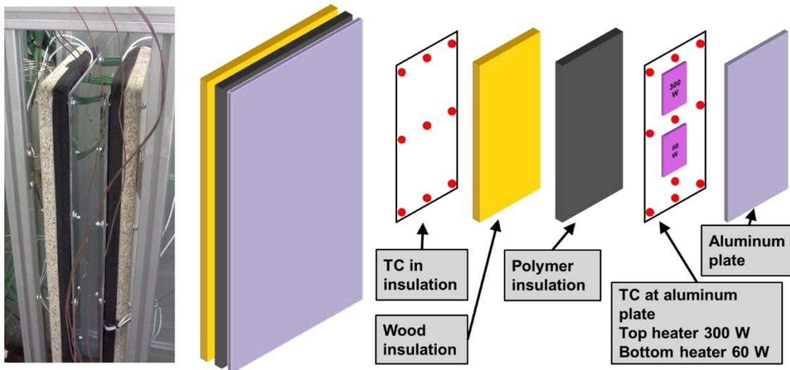
**Figure 8:** Experimental stand used for validation of the proposed cooling concept.
