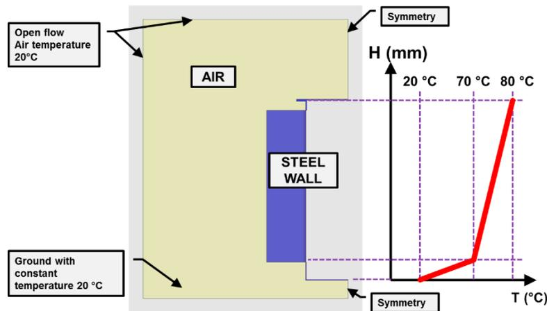
**Figure 9:** The model geometry and boundary conditions.
