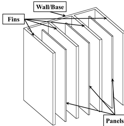
Figure 6: The schematic view of the concept of panels for increasing radiative heat transfer from fins.
