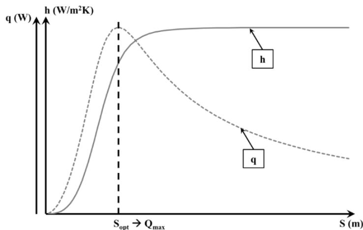
**Figure 3:** The dependence of the convective heat transfer coefficient and total heat transfer rate on fin spacing.
