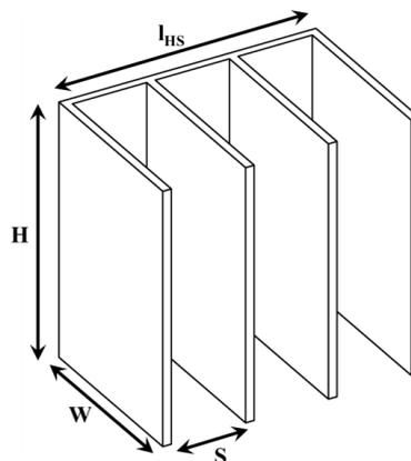
**Figure 2:** Basic configuration and parameters of the heat sink in a form of vertical plate with fins.
