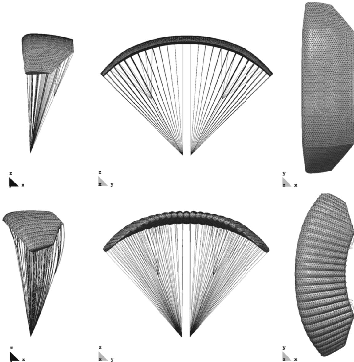
**Figure 3:** Three views of the initial (top) and computed (bottom) equilibrium configurations
