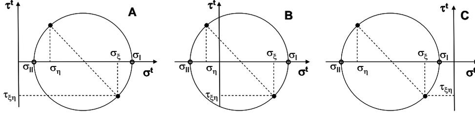
**Figure 1:** Trial membrane states: taut (A), wrinkled (B) and slack (C).
