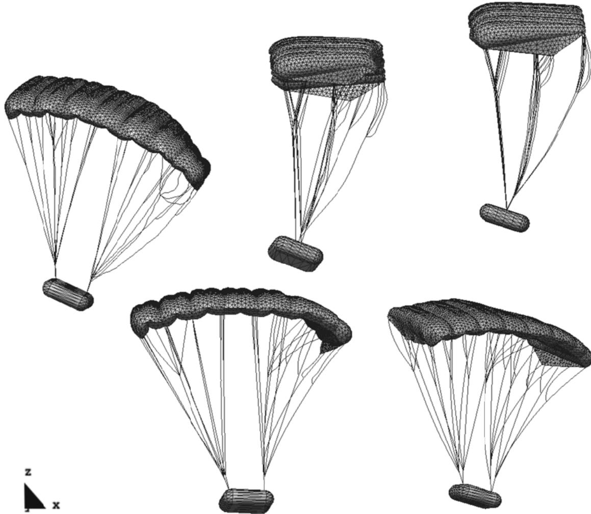
**Figure 6:** System configuration at five different instants of the maneuver simulation. In counterclockwise order: 3.6s, 15.6s, 19.1s, 19.9s and 23.2s
