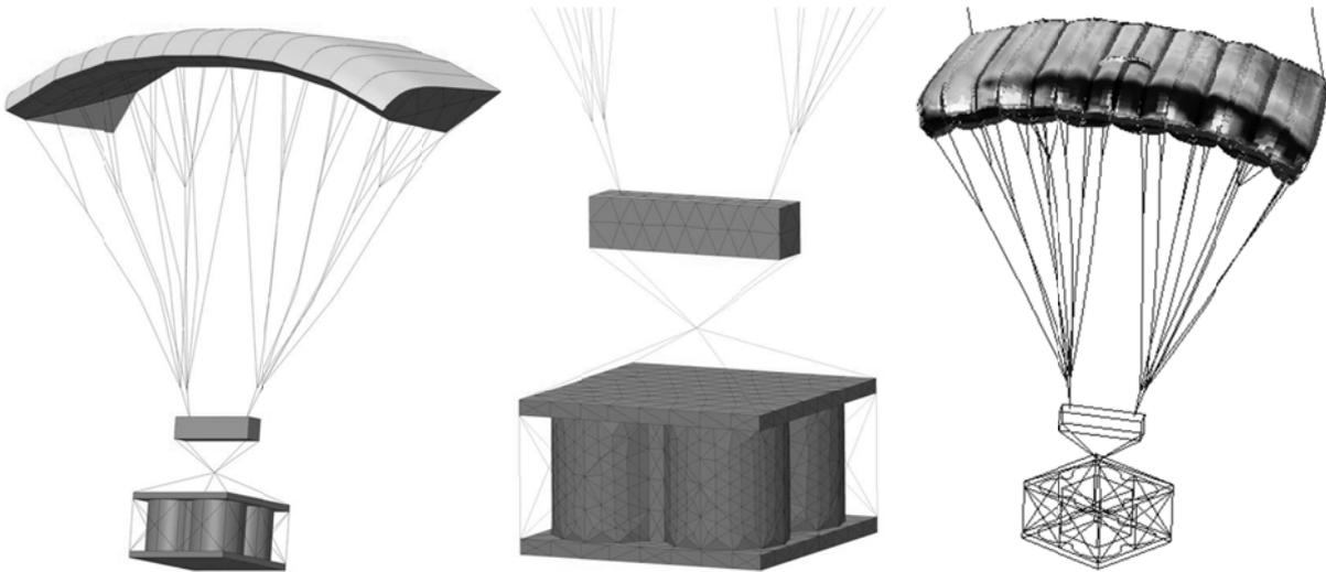
**Figure 7:** Original CAD model (left), detail of the payload modeled with rigid elements (center) and in-flight parachute deformed shape and pressure field (right)
