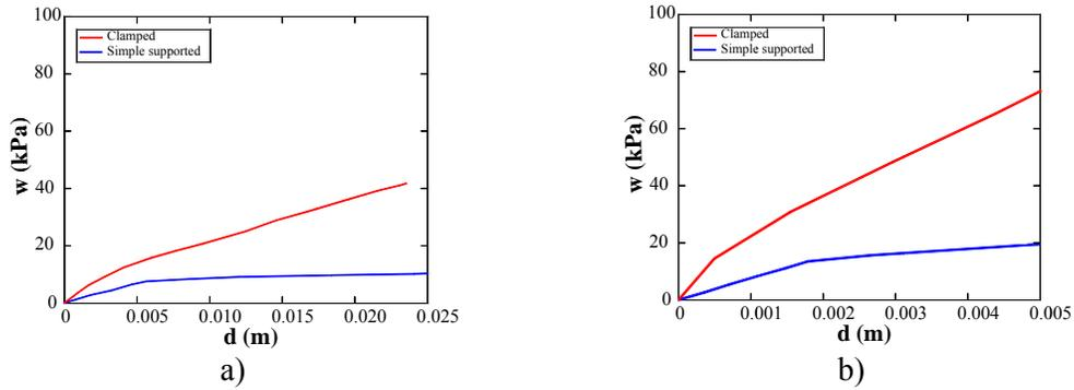
**Figure 6:** Distributed load vs. displacement in: a) square slab and b) rectangular slab
