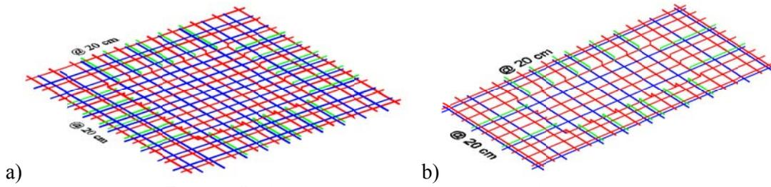
**Figure 5:** Steel reinforcement of slabs: a) square and b) rectangular
