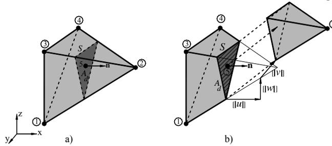
**Figure 2:** Finite element: a) discontinuity area and b) displacement jumps
