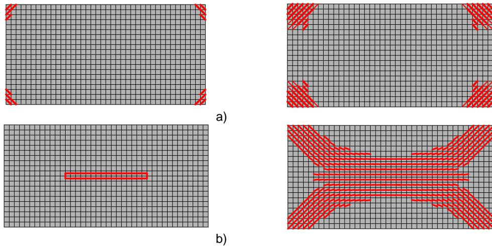
**Figure 10:** Cracking propagation of a simple supported rectangular slab on the: a) top and b) bottom surface
