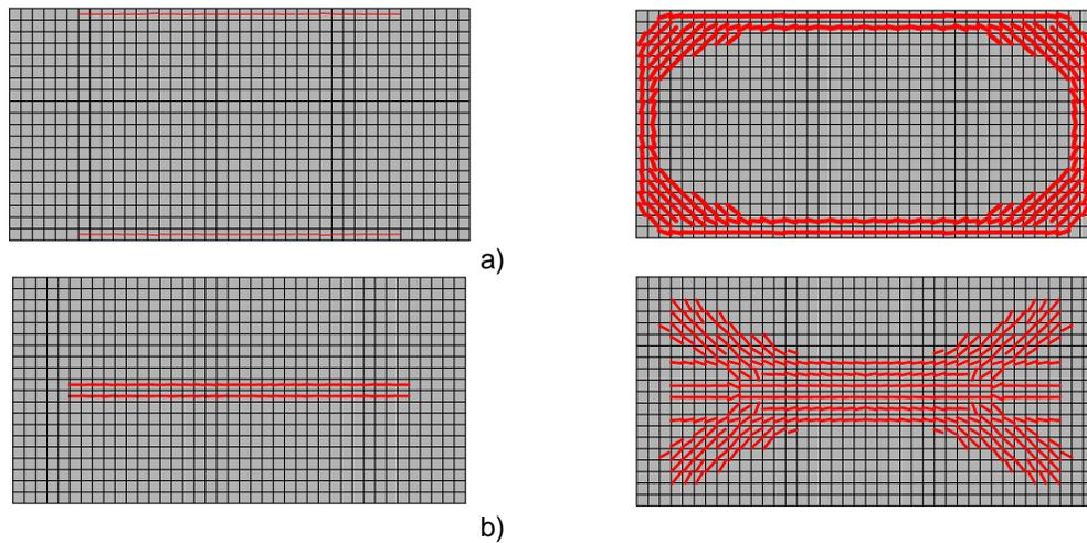
**Figure 9:** Cracking propagation of a fixed rectangular slab on the: a) top and b) bottom surface
