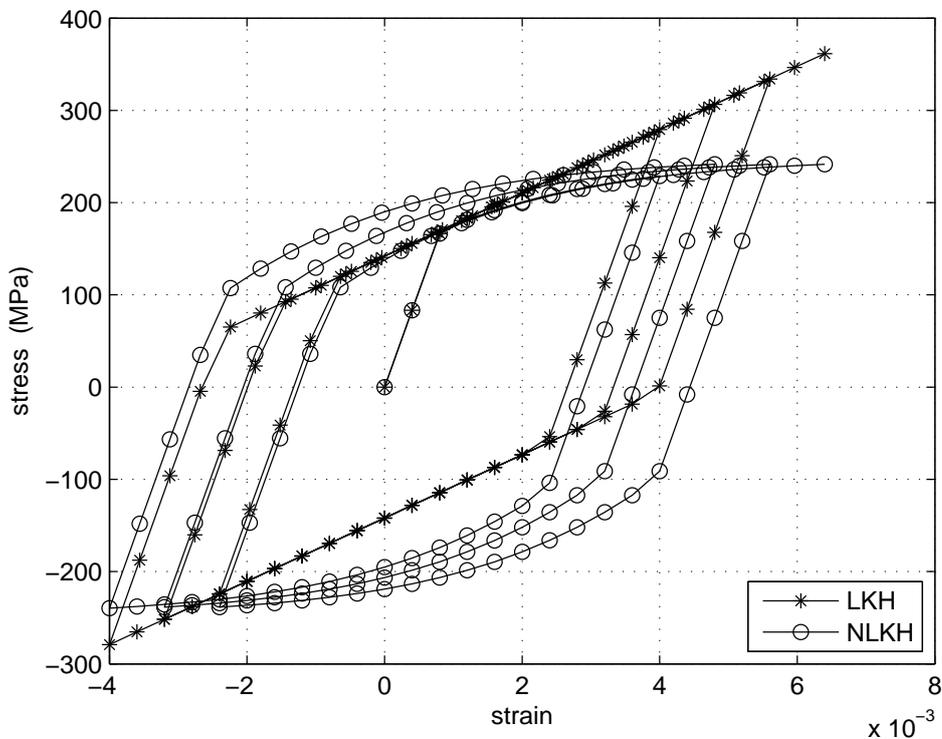
**Figure 2:** Cyclic loading condition in tension-compression for the steel X5CrNi 18-9 (loading program given in fig.1). Comparison between linear kinematic hardening (LKH) and nonlinear kinematic hardening (NLKH) in plasticity.
