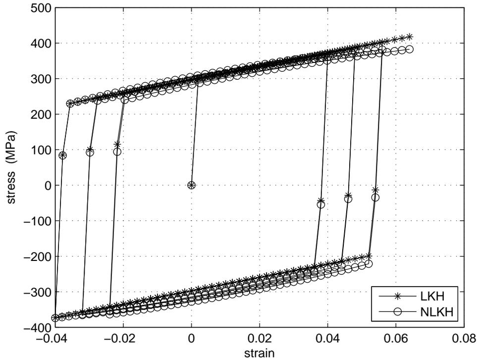
**Figure 5:** Cyclic loading conditions in tension-compression for the mild steel Ck 15 (loading program given in fig.1). Comparison between linear kinematic hardening (LKH) and nonlinear kinematic hardening (NLKH) in plasticity.
