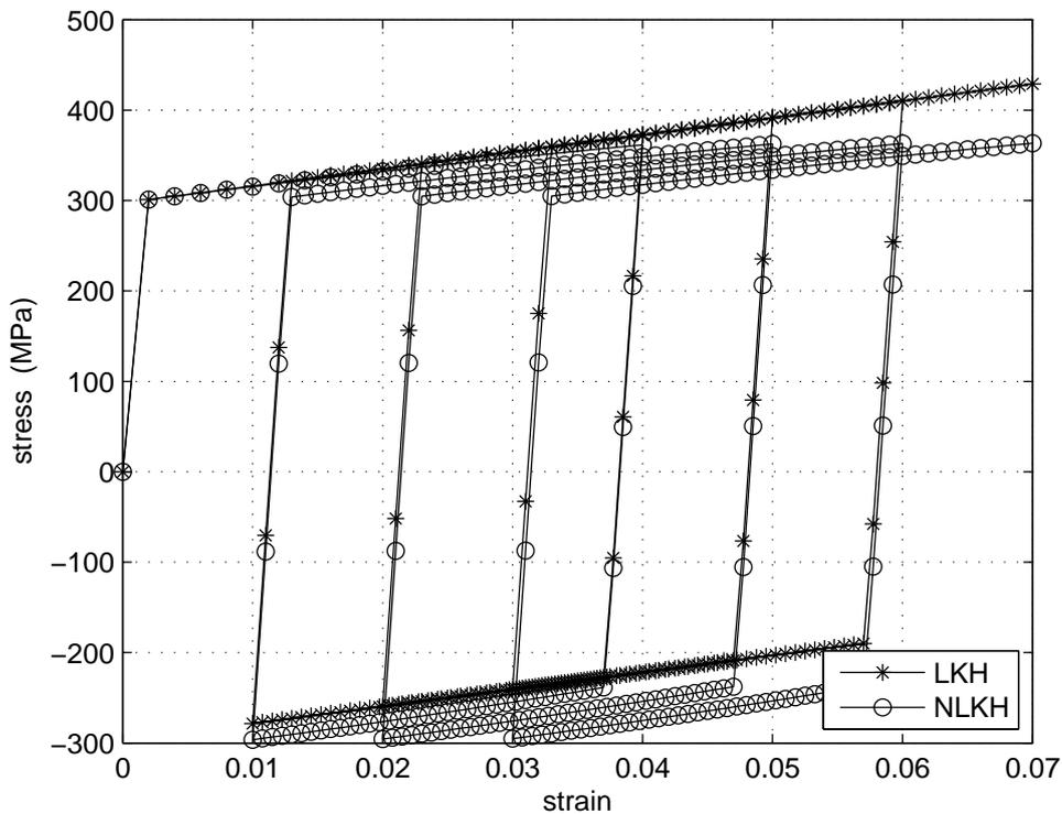
**Figure 6:** Cyclic loading conditions with increasing levels of loading for the mild steel Ck 15 (loading program given in fig.3). Comparison between linear kinematic hardening (LKH) and nonlinear kinematic hardening (NLKH) in plasticity.
