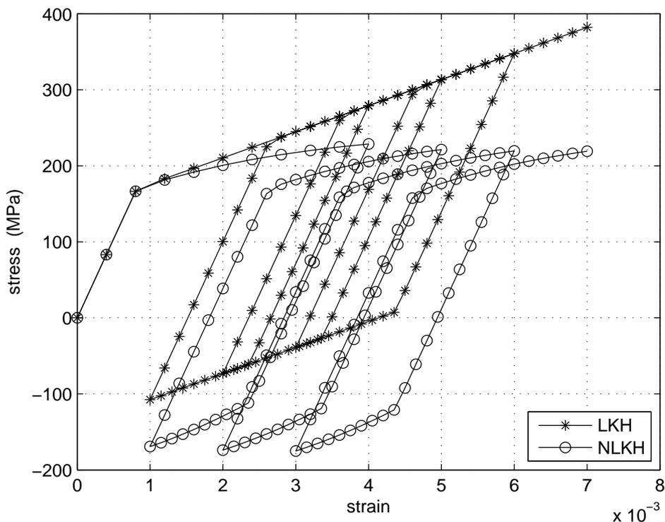
**Figure 4:** Cyclic loading condition with increasing levels of loading for the steel X5CrNi 18-9 (loading program given in fig.3). Comparison between linear kinematic hardening (LKH) and nonlinear kinematic hardening (NLKH) in plasticity.
