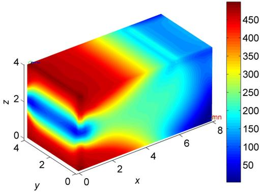
**Figure 2:** Distribution of von Mises stress  $\|\text{dev}(\sigma)\|_F$  at  $t_4$
