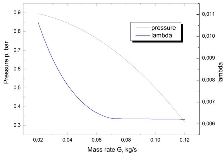
**Figure 2:** Drag coefficient versus the flow rate at  $IB = 0.15$  kATI
