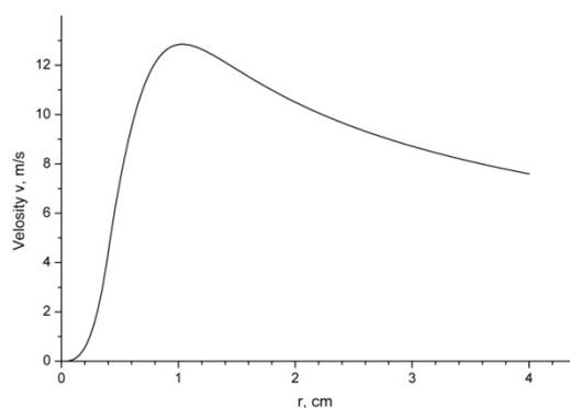
**Figure 5:** Distribution of the azimuthal velocity along the channel for  $G = 0.1$  kg/s  $IB = 0.45$  kATl
