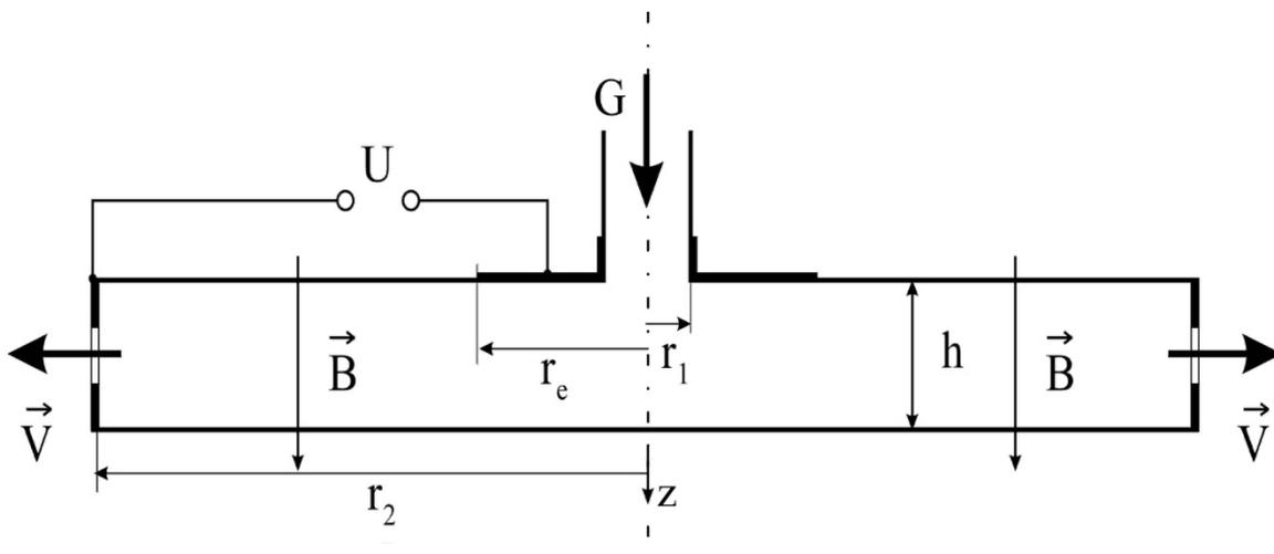
Figure 1: Scheme of the MHD cell
