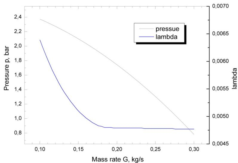
**Figure 3:** Drag coefficient versus the flow rate at  $IB = 0.45$  kATI
