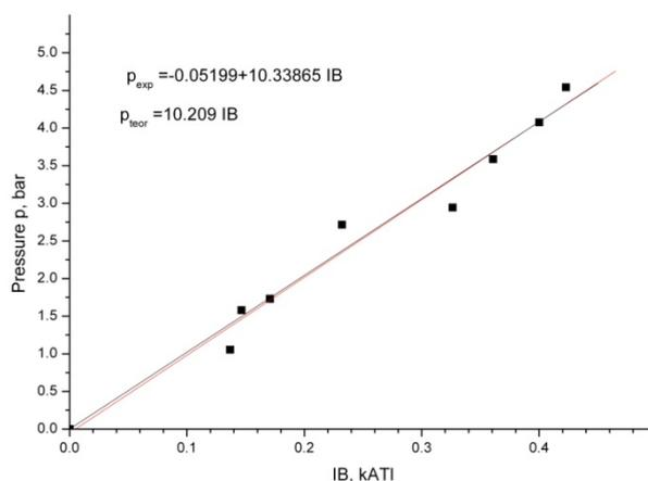
**Figure 7:** Comparative characteristics of the calculated and experimental data [2] in the regime with the zero flow rate. The solid curves show the calculated results; the squares are the experimental data
