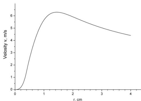
**Figure 4:** Distribution of the azimuthal velocity along the channel for  $G = 0.1$  kg/s  $IB = 0.15$  kATl
