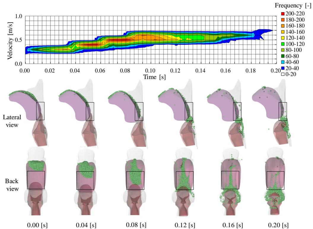
Figure 3 Velocity profiles and configuration of thickener
