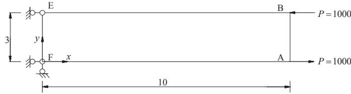
**Figure 3:** Cantilever beam under pure bending moment
