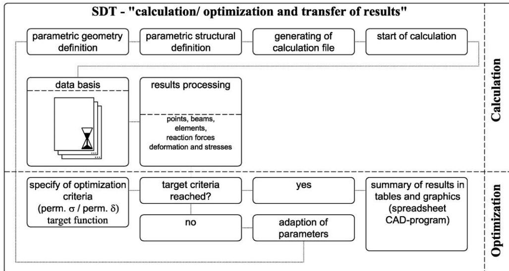
Figure 5: SDT – calculation / optimization and transfer of results [5]
