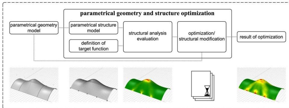
**Figure 12:** The use of parametric tools for geometry definition and analysis
