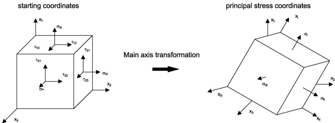
**Figure 11:** Principal stress transformation of the stress tensor, adapted illustration by [13]
