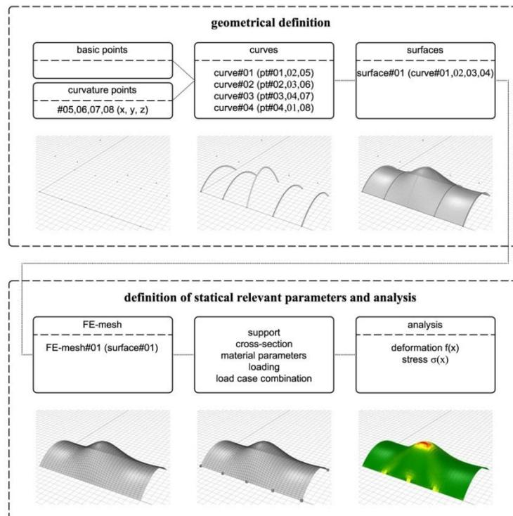
Figure 4: Parametric tools for geometry definition and analysis [5]
