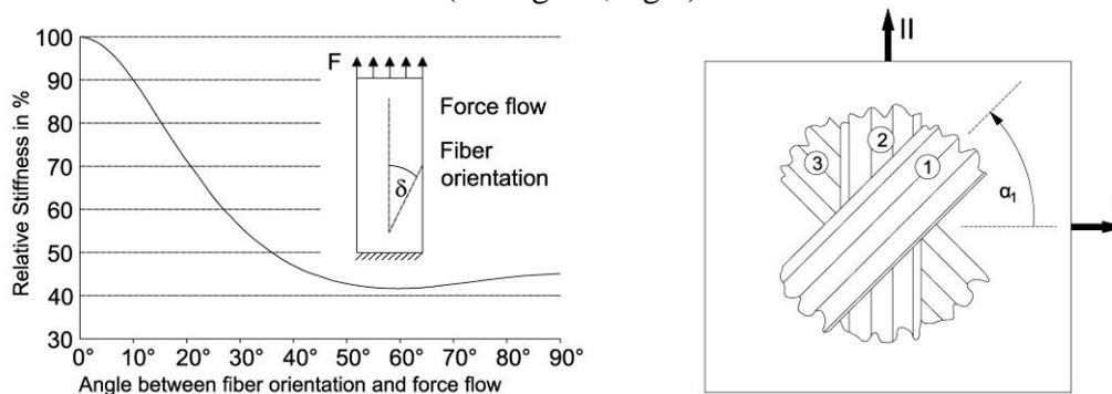
**Figure 10:** Left: relationship between fiber orientation and stiffness [13]; right: multilayer laminate [14]
