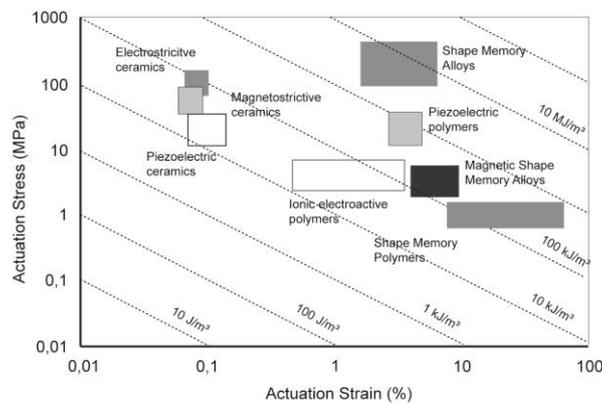
Figure 3: Stress-strain diagram of smart materials [3]
