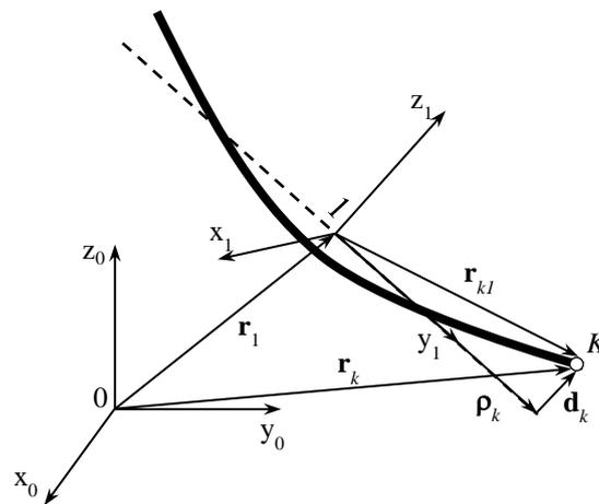
**Figure 1:** Position of an arbitrary point  $K$  of a flexible body
