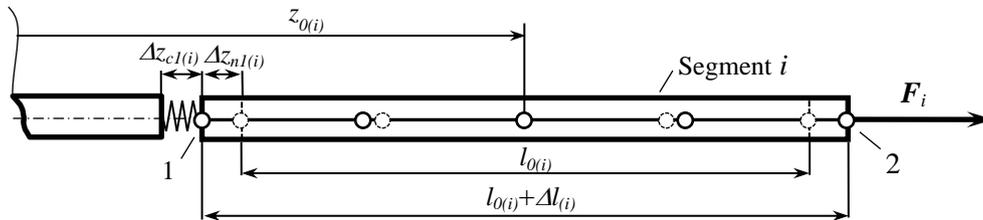
**Figure 5:** Calculation of the initial positions of the segment  $i$  with use of the static results
