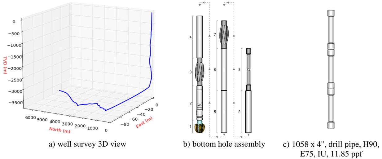
**Figure 6:** Three-dimensional view of the well bore centerline and outline of the drill string in the example
