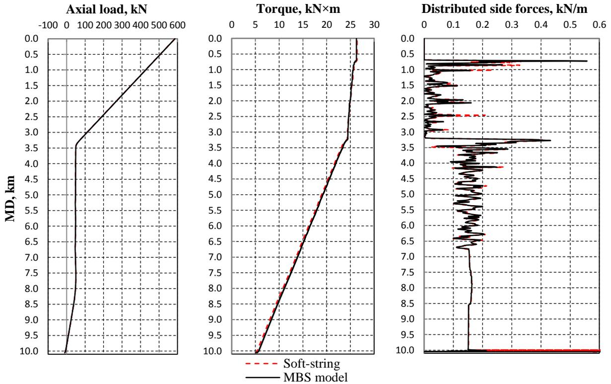
**Figure 9:** Comparison of results obtained by using soft-string and multibody system approach
