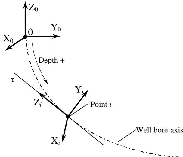
**Figure 3:** Natural coordinate system in the point  $i$  on the centerline of a well bore
