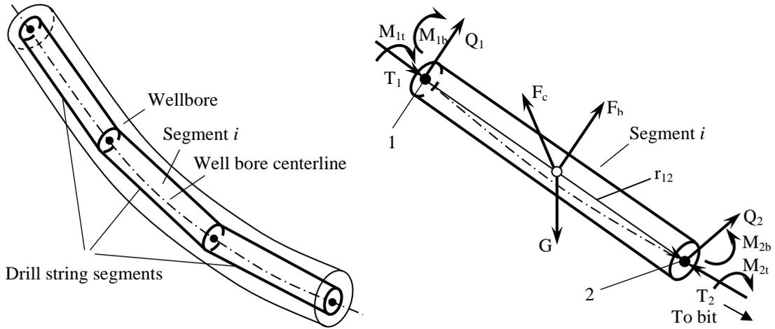
**Figure 4:** Arrangement of end points of the drill string on the wellbore centerline and the forces acting on segment  $i$ .
