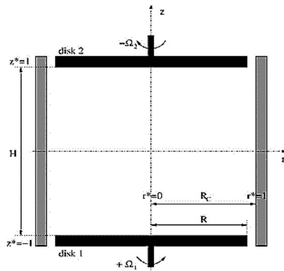
Figure 1. Sketches of the cavity with relevant notation
