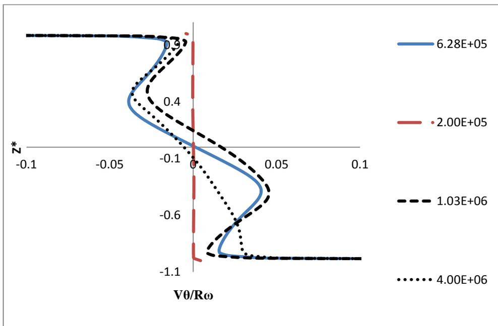
**Figure 3.** Axial profiles of the tangential velocity component for  $\Gamma = -1$ ,  $r^* = 0.476$  at different  $Re$
