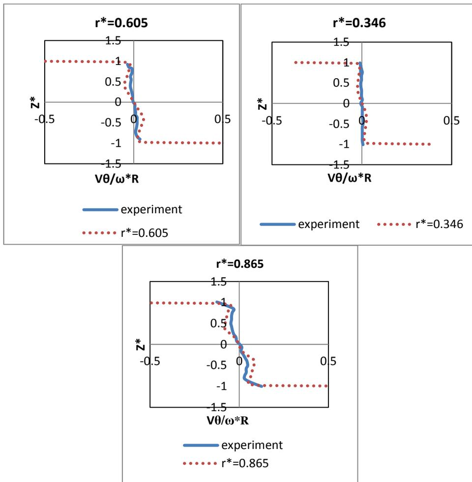
**Figure 2.** Axial profiles of the tangential velocity component for  $\Gamma = -1$ ,  $Re = 6.28 \times 10^5$  and  $G = 1.8$
