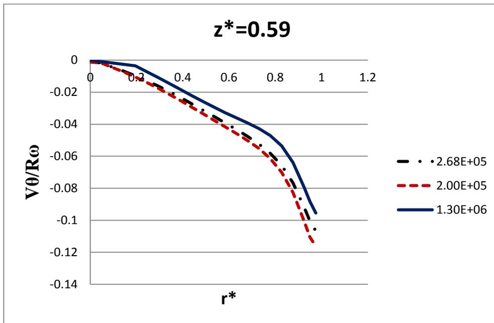
Figure 4. Radial profiles of the tangential velocity component in the smooth disk case for  $\Gamma = -1$ ,  $G = 1:8$  and four Reynolds numbers at different axial locations
