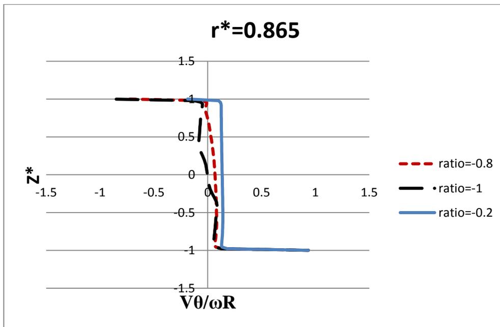
Figure 5. Axial profiles of the tangential velocity component in different rotation ratio
