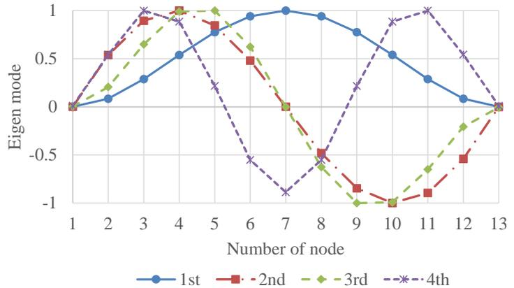
Figure 3: Mode shapes in vertical y-directions
