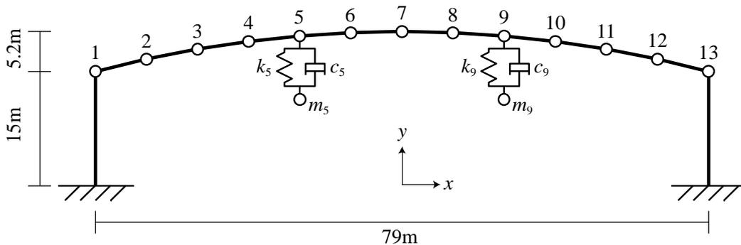
Figure 2: Arch-frame model with attached TMDs at the 5<sup>th</sup> and 9<sup>th</sup> nodes.
