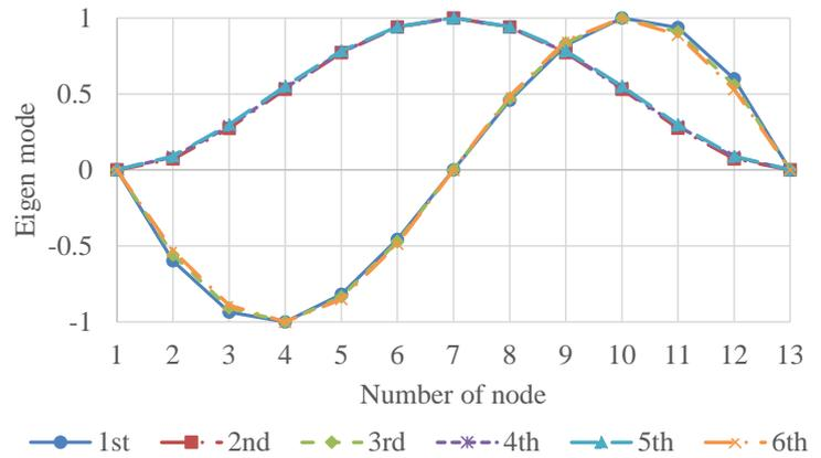
Figure 5: Real part of mode shapes in vertical y-directions
