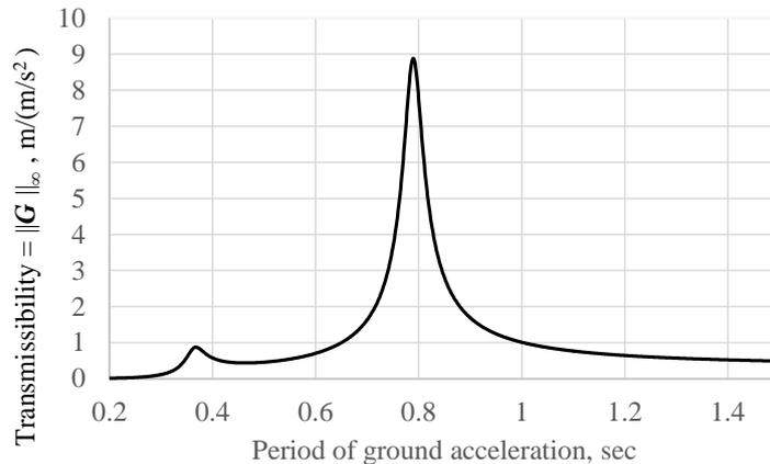
Figure 4: Frequency response function of the main structure
