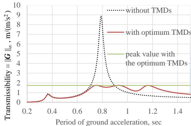
Figure 6: Comparison of frequency response function
