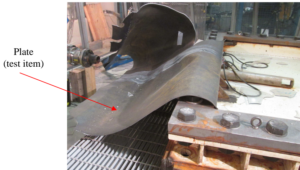
Figure 4: Photograph showing the complete tearing on three sides of the plate for the test No. 5
