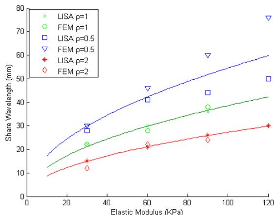
**Figure 4:** Simulated shear wavelengths for different elastic modules and material densities. Analytical solutions are given by solid lines
