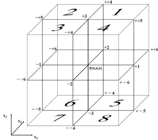
**Figure 1:** Eight elementary discretisation scheme used for wave propagation modeling in the LISA 3D.
