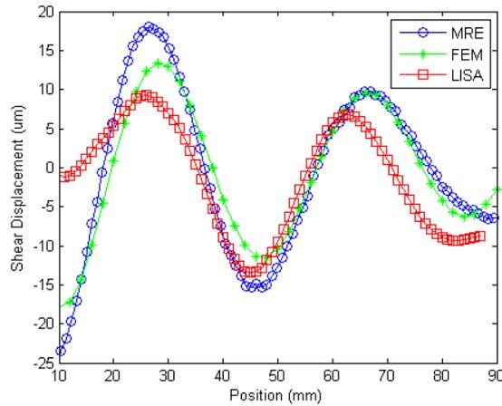
**Figure 3:** Comparison of the simulated FE and LISA displacement waveforms the relevant MRE measurement for the cylindrical agar gel phantom.
