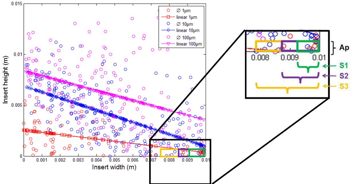
**Figure 2:** Example of the results showing the particle impingement a) on the insert and b) on the different tool-chip contact areas ( $S_1$ ,  $S_2$ ,  $S_3$ ), for  $V_c = 5026$   $m/min$  and  $P_{inlet} = 0.1$   $MPa$  inlet pressure, for  $45^\circ$  canalization orientation.
