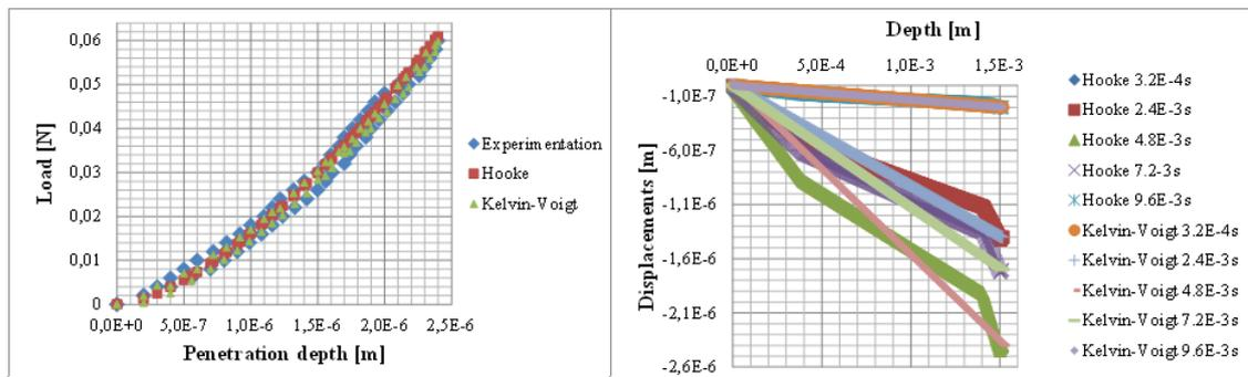
Figure 6: (left) Comparison between numerical and experimental displacement curves (right) Displacements of the solids
