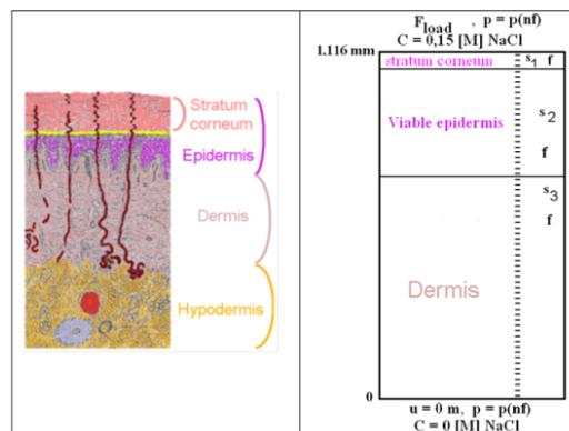
Figure 1: Schematic view of the cross-section of human skin (left) and of the skin specimen (right) showing the finite difference mesh and the boundary conditions
