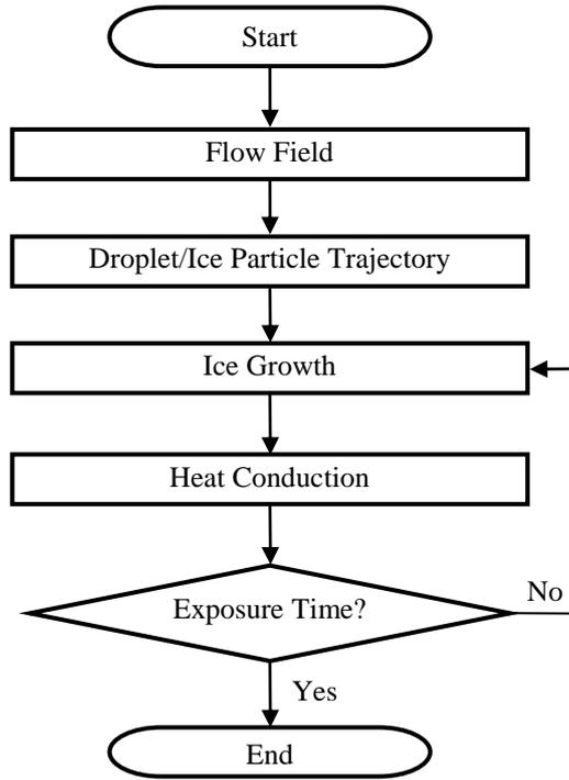
**Figure 1:** Algorithm of ice accretion simulation
