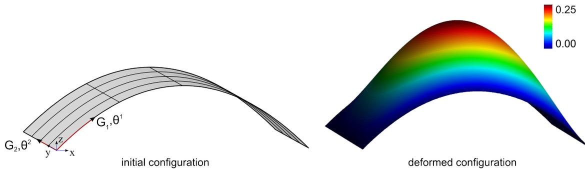
Figure 3: Initial and deformed configuration of the benchmark for CSM
