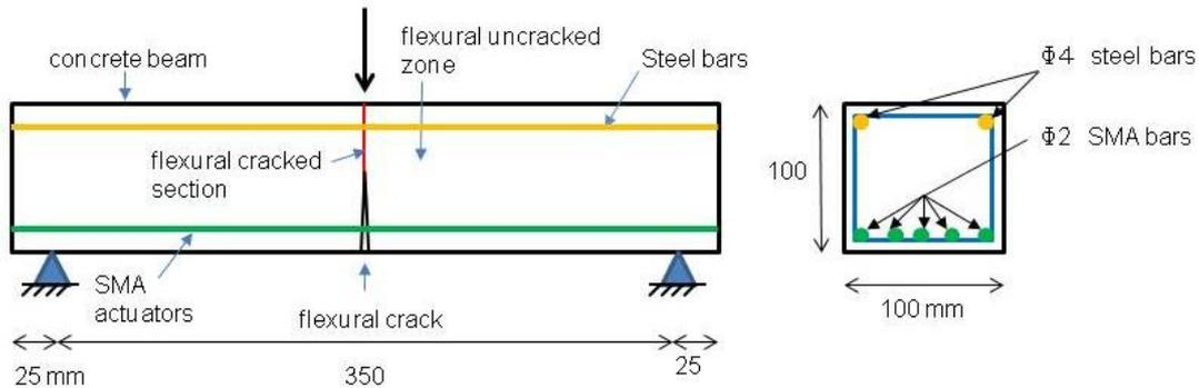
**Figure 1:** Schematic representation of reinforced concrete beam with SMA actuators.
