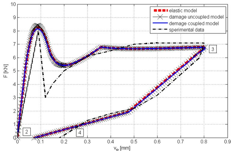
**Figure 3:** Experimental and numerical mid-span displacement versus load graph. (specimen L1 [1]).
