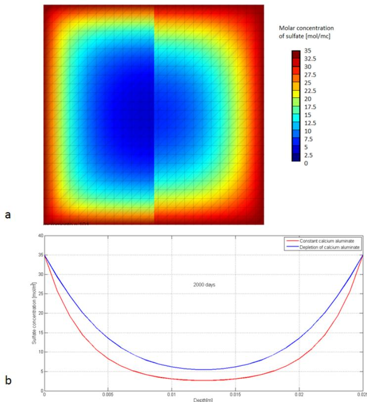
**Figure 1:** a) Molar concentration of sulfate in the cross section of the specimen at 2000 days (right part: considering depletion of aluminates, left part: neglecting depletion of aluminates), b) profiles of molar concentration of sulfate along the middle line.
