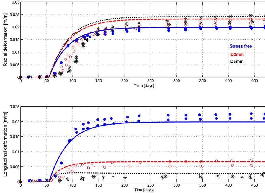
**Figure 3:** Transversal and longitudinal strains of specimens subject to DEF in stress-free conditions and under restraint: experimental points from [8] and numerical prediction.
