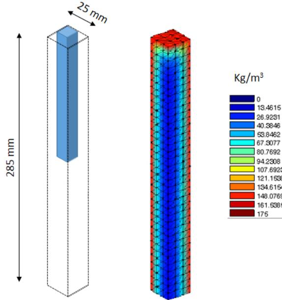
**Figure 2:** Ettringite distribution at 2,000 days considering depletion of aluminates.
