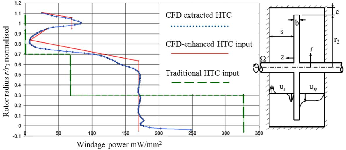
**Figure 4:** Radial distribution of rotor windage in a typical turbine rotor-stator cavity
