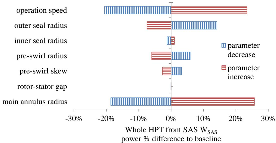
**Figure 6:** Percentage impact of each SAS design variation on the power loss of the whole HPT front SAS. The baseline whole SAS power loss is the addition of the individual feature powers, presented in Figure 5.
