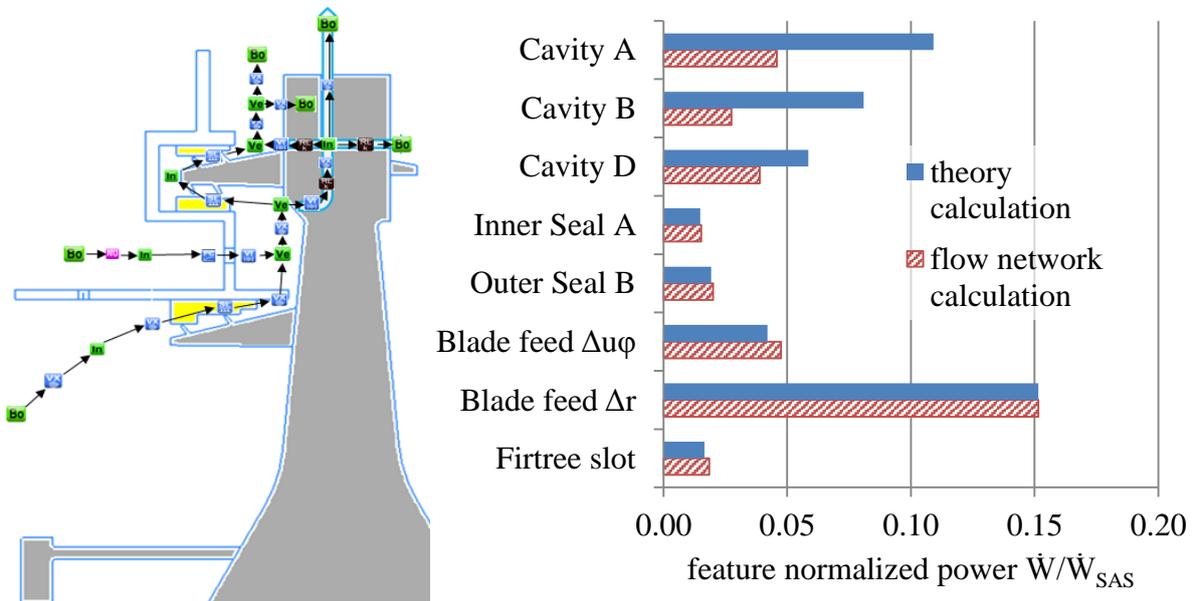
**Figure 5:** 1D flow network model of the HPT SAS (left); and comparison of the front HPT SAS power losses calculated with the enhanced flow network model and the theoretical approach, normalized with  $\dot{W}_{SAS}$  (right)
