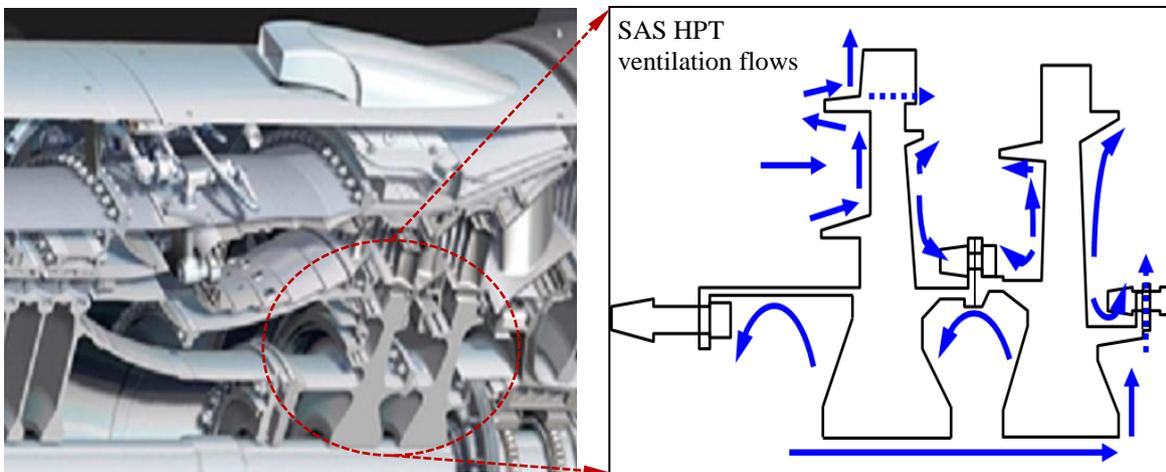
**Figure 1:** Aero engine 2-stage HPT cutaway (left) & SAS disc cavity ventilation flows (right). Courtesy of Rolls-Royce Deutschland
