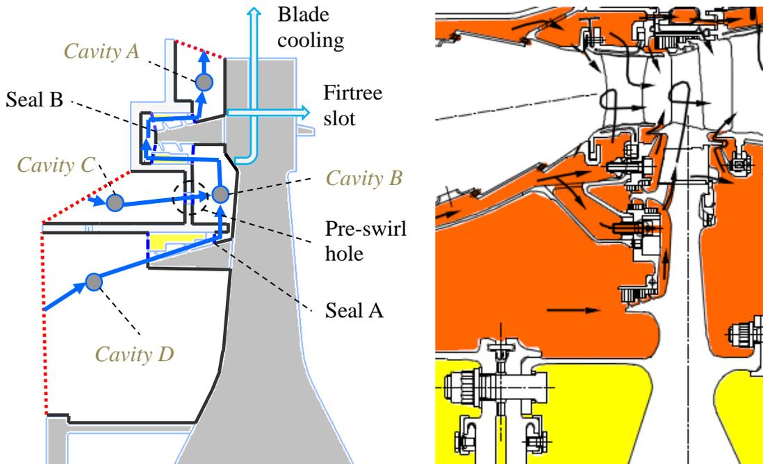
**Figure 2:** Configuration of the HPT front application case SAS features (left); and diagram of the SAS flows in a realistic turbine geometry (right)
