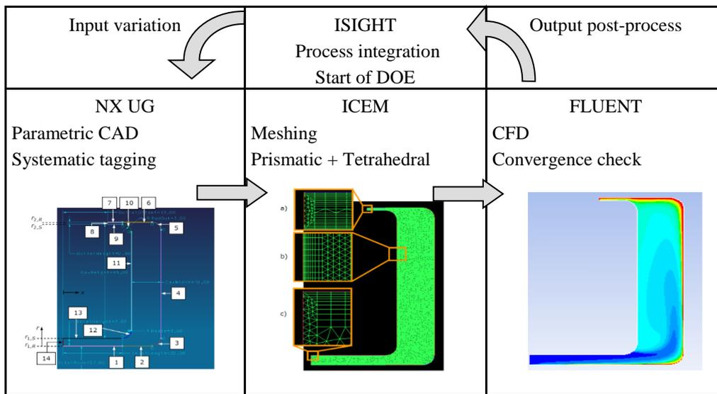
**Figure 3:** Parametric CFD workflow and coupled applications
