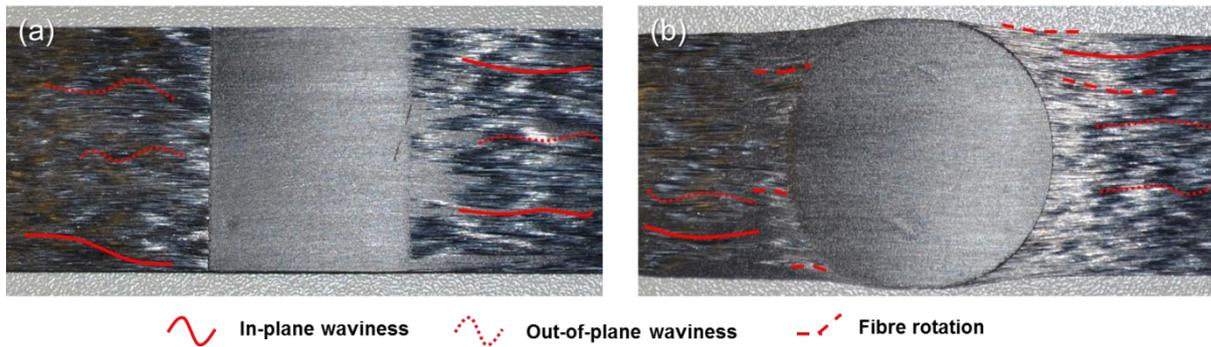
**Figure 2:** Observed defects after the joining process.
