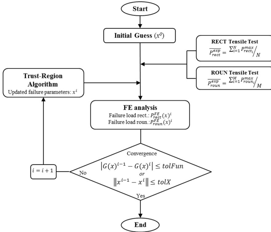
Figure 3: Scheme of the calibration process.
