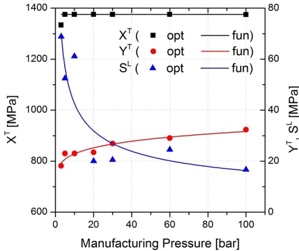
**Figure 4:** Strength parameters for different forming pressures. Output of the optimization routine (opt) and correlation of proposed functions (fun) are shown.
