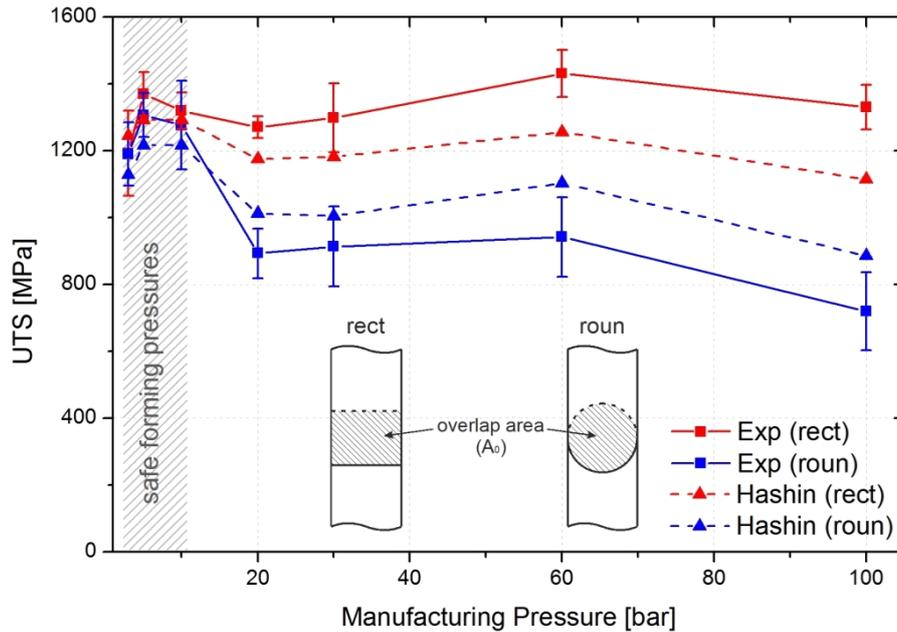
**Figure 1:** UTS dependence on forming pressure of the SLJs. The UTS is defined as the maximum tensile load divided by the cross-sectional area of one adherend. Hashin predictions are also shown.
