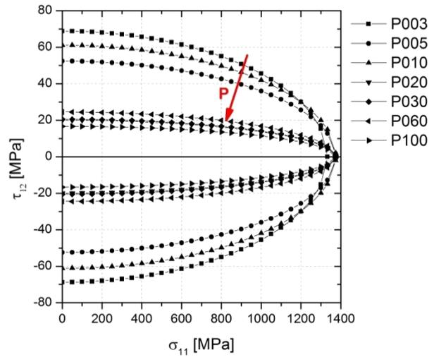
**Figure 5:** Failure envelope variation with forming pressure. Tension-shear plane.
