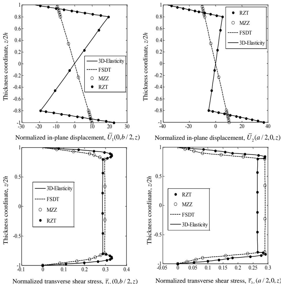
**Figure 4.** Laminate L2,  $a/2h=6$ : through-the-thickness distribution of normalized in-plane displacement,  $\bar{U}_\alpha = (10^4 D_{11}/q_0 a^4) U_\alpha^{(k)}$  and normalized transverse shear stress,  $\bar{\tau}_{\alpha z} = (2h/q_0 a^2) \tau_{\alpha z}^{(k)}$ . The FSDT solution is obtained with  $k_x^2 = 0.0242$ ,  $k_y^2 = 0.0225$ .
