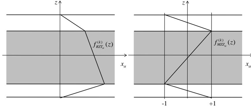
Figure 2. Comparison on the through-the-thickness distribution of zigzag functions.
