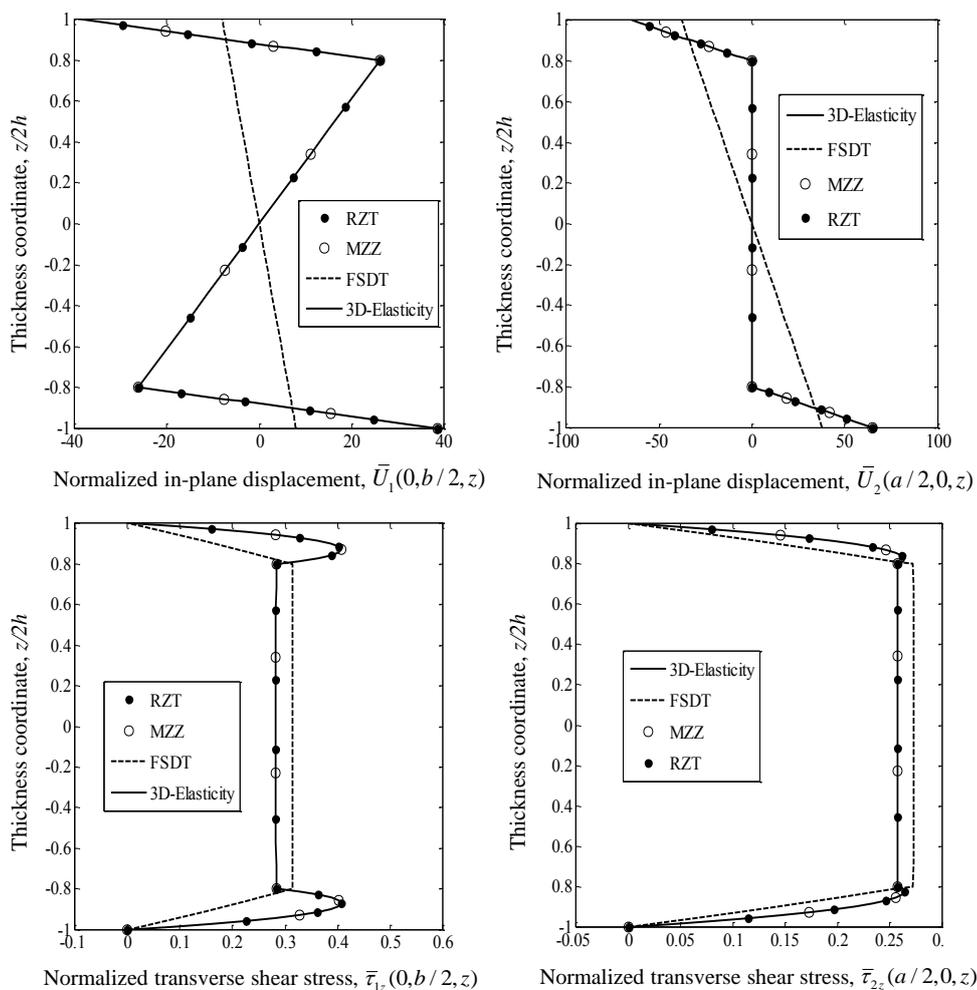
**Figure 3.** Laminate L1,  $a/2h=6$ : through-the-thickness distribution of normalized in-plane displacement,  $\bar{U}_\alpha = (10^4 D_{11}/q_0 a^4) U_\alpha^{(k)}$  and normalized transverse shear stress,  $\bar{\tau}_{\alpha z} = (2h/q_0 a^2) \tau_{\alpha z}^{(k)}$ . The FSDT solution is obtained with  $k_x^2 = k_y^2 = 0.022$ .
