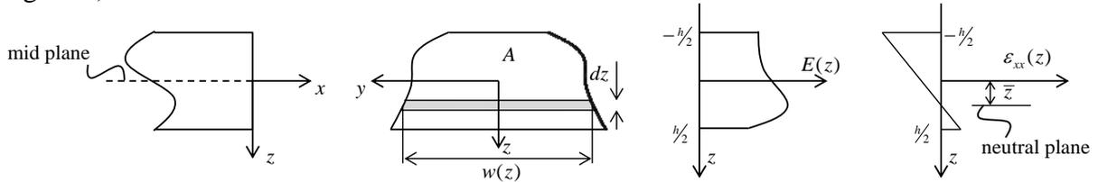
**Figure 3:** Homogenization of non-symmetric FGM beams
