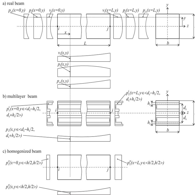
**Figure 1:** FGM beam with spatial variation of material properties
