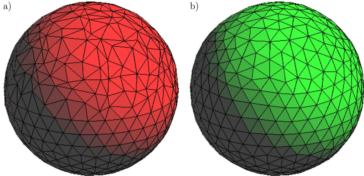
**Figure 5:** Smoothing of a surface mesh (with 816 elements) over a unit sphere: (a) original mesh (perturbed on the top hemisphere), (b) smoothed mesh.
