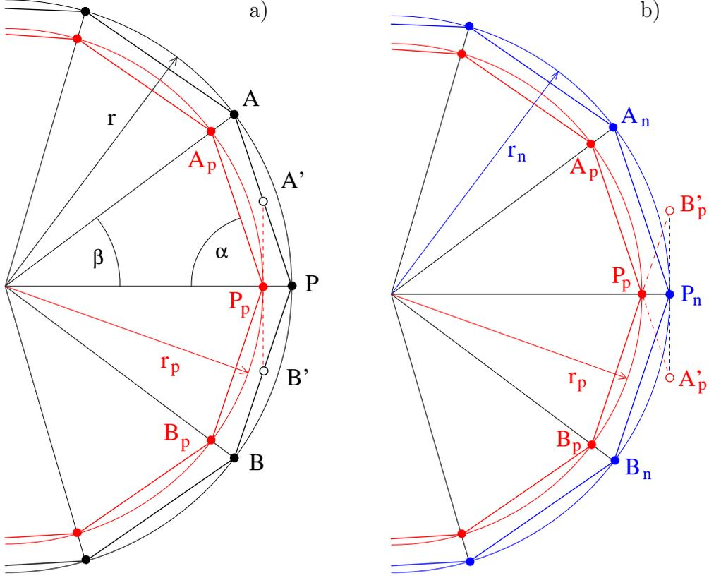
**Figure 1:** Two subcycles of smoothing: (a) shrinkage (using positive weight  $\lambda$ ), (b) expansion (using negative weight  $\mu$ ).
