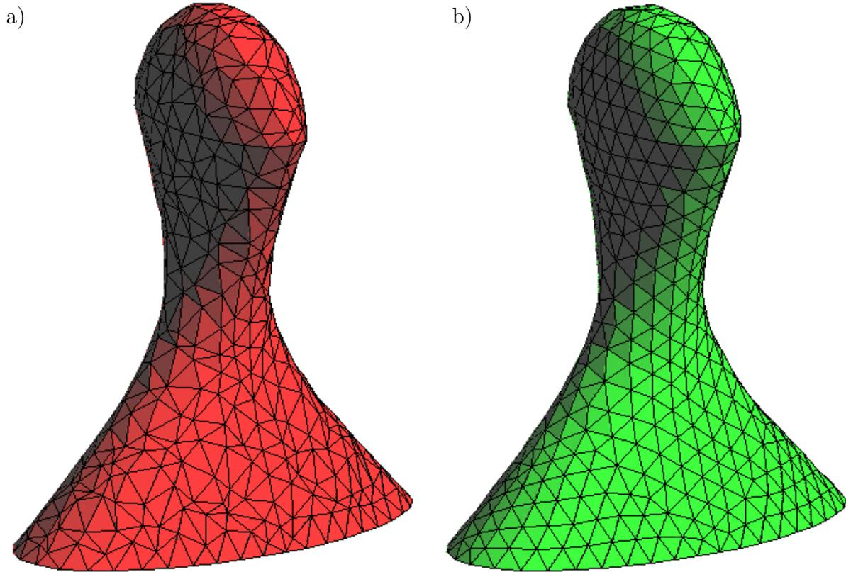
**Figure 7:** Smoothing of a surface mesh (with 1426 elements) over a pawn-like figure: (a) original mesh, (b) smoothed mesh.
