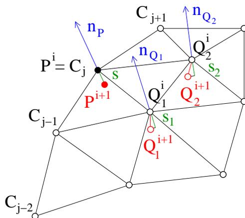
**Figure 4:** Geometrical setup for the assessment of shrinkage at curve node  $P$  of an open surface.
