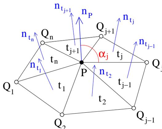
**Figure 2:** Geometrical setup for the evaluation of smoothing weights for inner node  $P$  on a surface.
