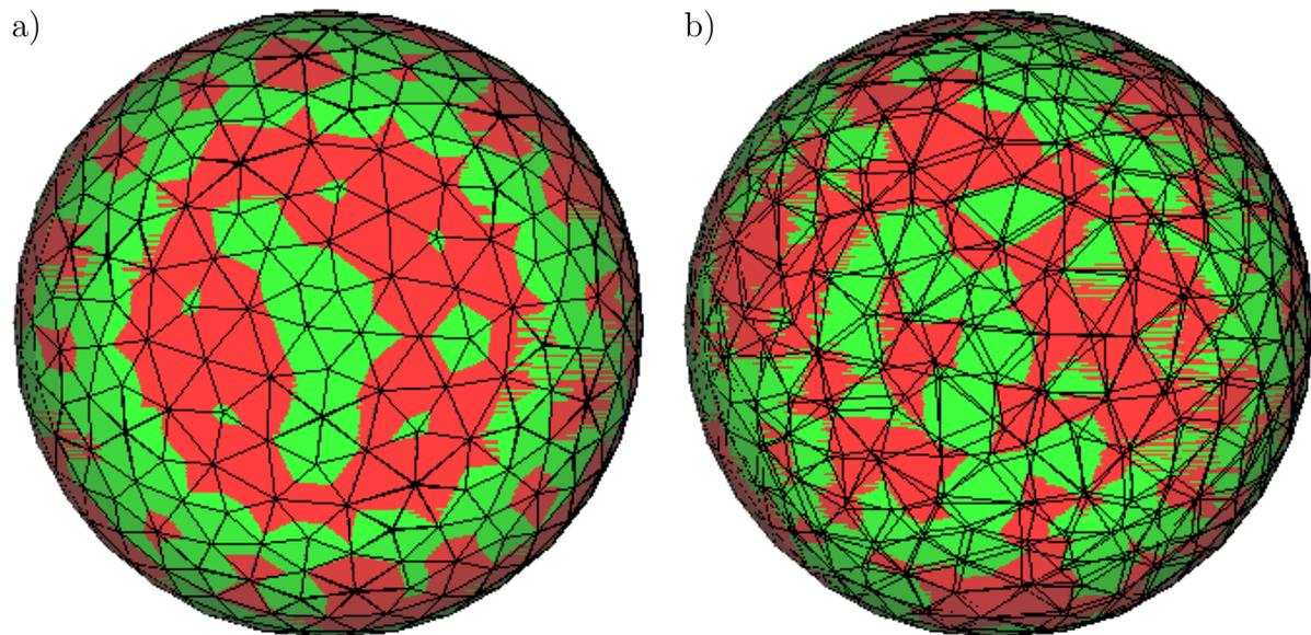
**Figure 6:** Overlay of original and smoothed mesh (with 816 elements) on a unit sphere: (a) over unperturbed hemisphere, (b) over perturbed hemisphere.
