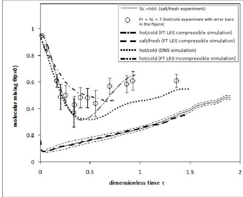
**Figure 2:** Hot-cold water channel splitter plate experiment of Rayleigh-Taylor instability with experimental measurements [23], the nearly DNS incompressible simulation, our own front tracking incompressible simulation using lower grid resolution, a compressible front tracking simulation reported earlier [20] and fresh-salt water channel experiments and simulations. The very large Schmidt number  $Sc = 560$  makes this case infeasible to simulate without the use of front tracking.
