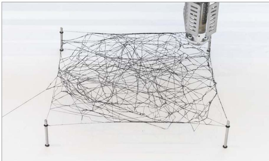
Figure 6: Example of 300mm x 300mm flat mesh.
