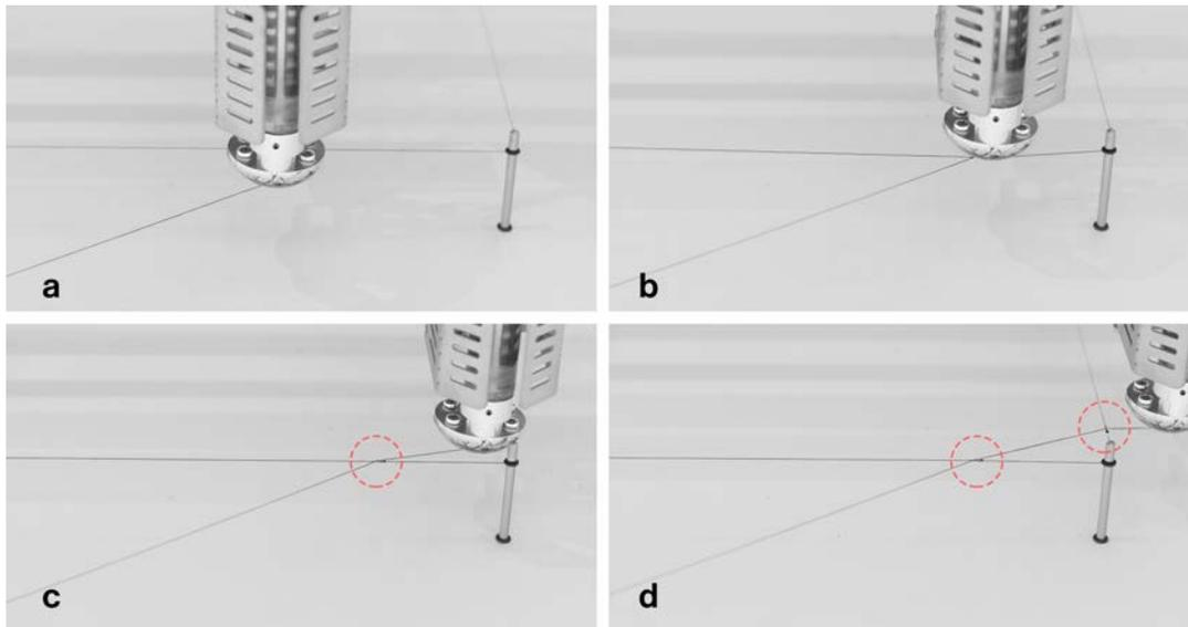
Figure 4: Image sequence showing the creation of two anchor points on a thread frame.
