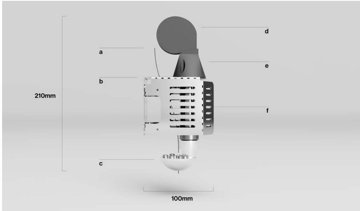
Figure 1: Render of the end-effector and its components. (a) Heat-bonding thread; (b) Stainless steel guard; (c) Aluminum nozzle; (d) Fan; (e) Fan Adapter; (f) Heater.
