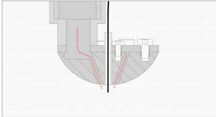
Figure 2: Section view of the nozzle. The red arrows indicate the air flow within the nozzle.
