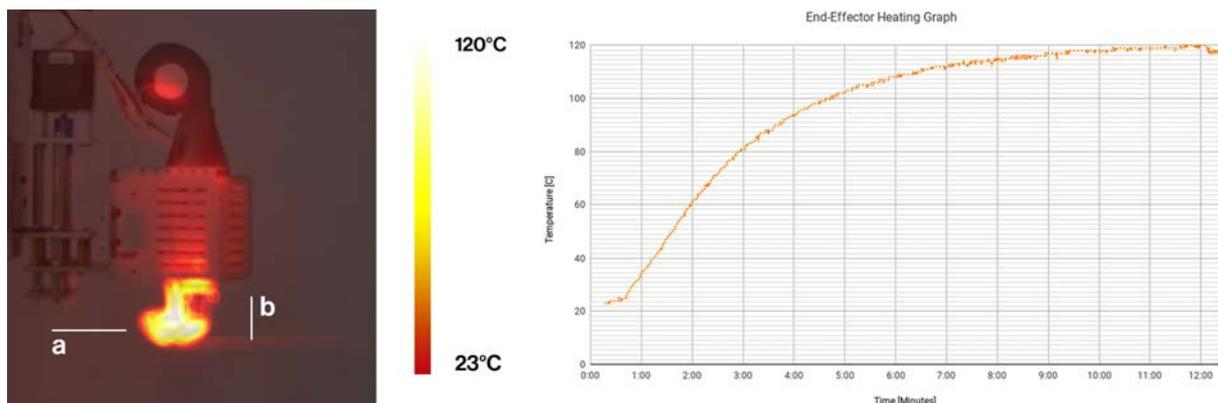
Figure 3: IR heatmap showing heat distribution on nozzle (a) and thread (b). Graph (right) shows heating curve of End-Effector at room temperature.
