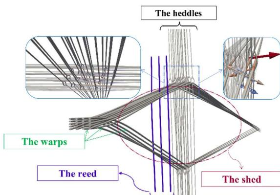
Figure 1 : Simulation model at shedding phase showing frictional contact interactions
