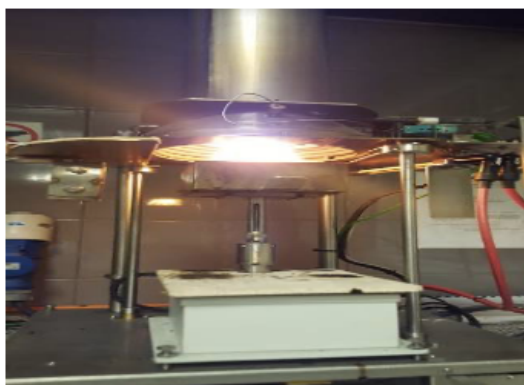
Figure 2. MLC apparatus set at 35 \text{ kW/m}^2 .
