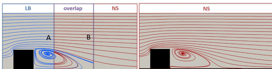
Figure 1 Comparison between NS/LB dual model (right) and single NS model. Streamlines around a 3D wall mounted cube on the central vertical plane. LB streamlines (blue), NS streamlines (red).
