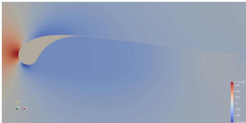
**Figure 1:** Pressure Poisson's equation is solved in a sub-domain of the computational field to avoid connectivity between suction side and pressure side.
