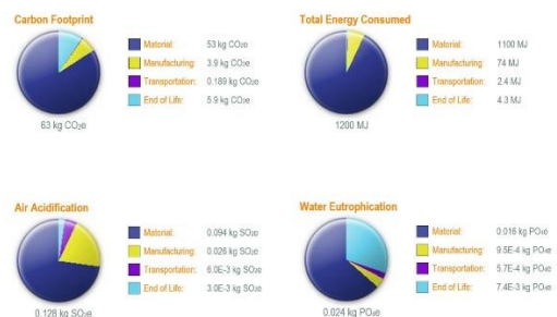
Figure 2. LCA results adopting CML methodology in SolidWorks 2015
