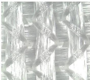
Fig.1 Warp knitted fabric structures
