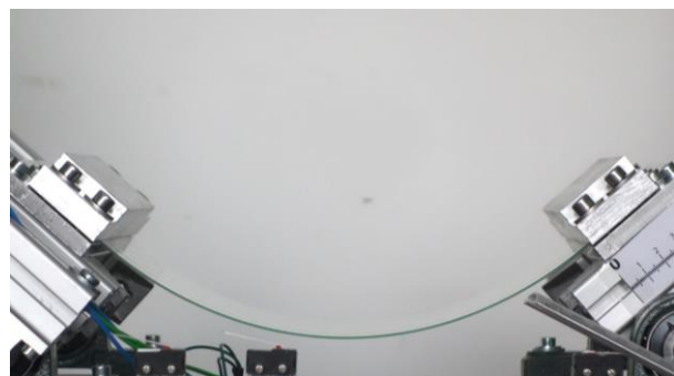
Figure 2: thin glass during uniaxial bending test
